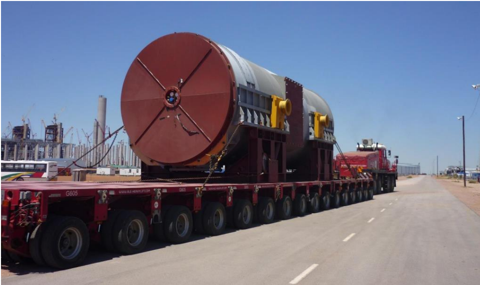
Figure 6: Heavy haulage truck with 16-axle hydraulic trailer transporting a 360 ton generator (source: ALE)
