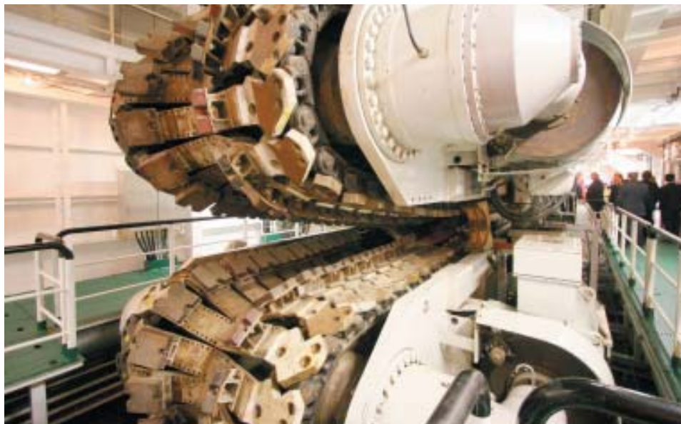
The tensioners keep the pipe stationary and prevent buckling
