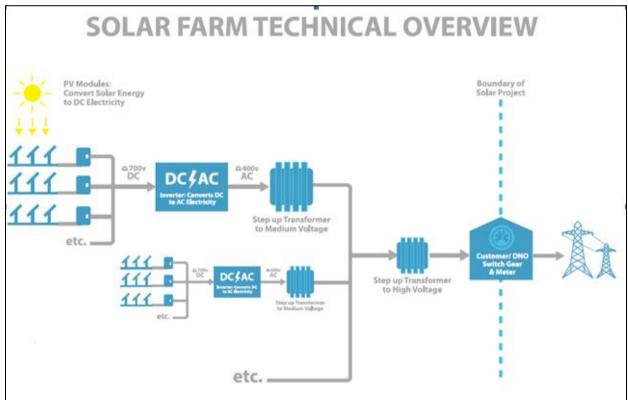
Figure 3.4: General Functional Overview of a Typical Solar Project showing Key Components
