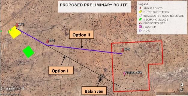
Figure 2.3: The proposed preliminary route from AP1 to AP3 showing the angle at AP2.
