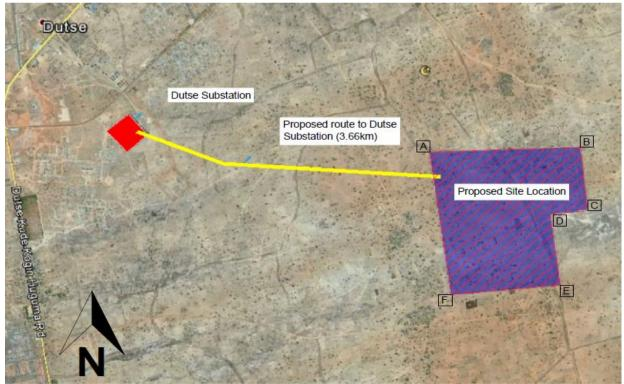
Figure 3.6: Project Site (Dutse-2) and Proposed Route for 132kV Overhead Line
