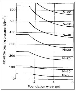
Fig: 6: Settlement of footing from standard penetration resistance
