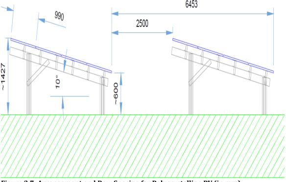
Figure 3.7: Arrangement and Row Spacing for Polycrystalline PV (in mm)
