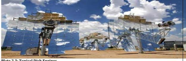
Plate 2.3: Typical Dish Engines
