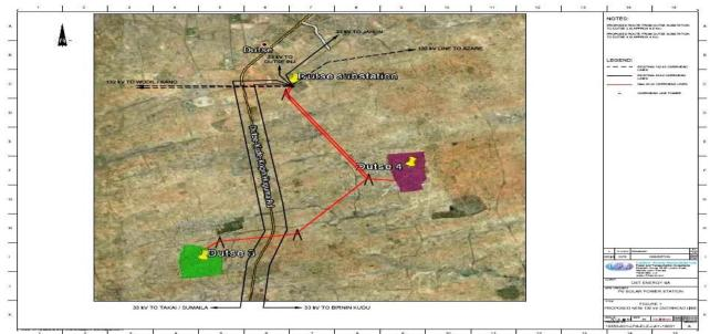
Figure 2.1: Map Showing Layout of Dutse 3, Dutse 4, Dutse Substation and Proposed Transmission Route.
