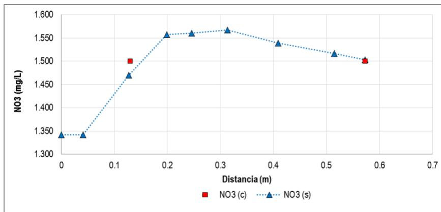
**Illustration 5-81.** Calibration results of nitrates in simulation section No. 2
