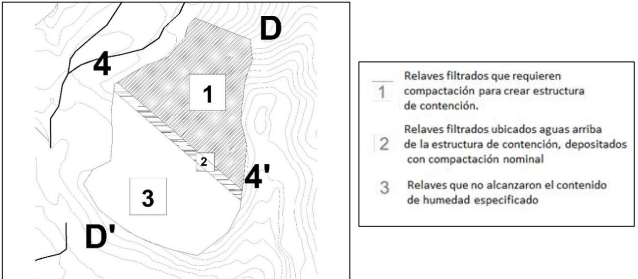
**Illustration 5-7.** Recommended compaction areas for tailings deposit No. 4.
