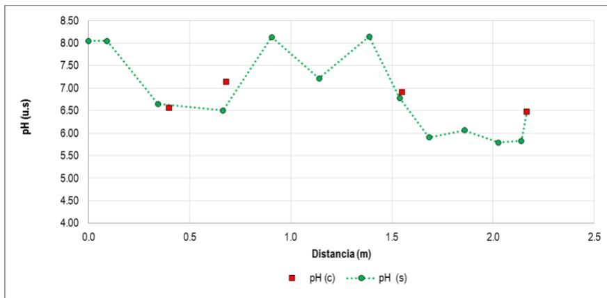
Illustration 5-92. Results calibration of the pH in the simulation section N ° 1
