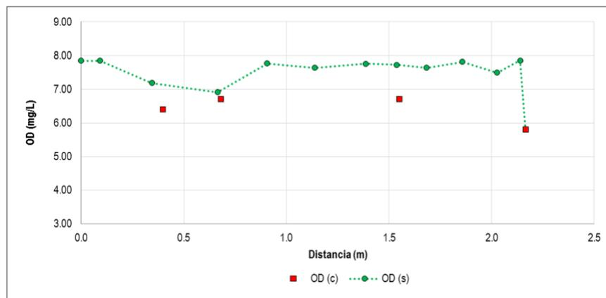
**Illustration 5-74.** Results calibration of the dissolved oxygen in the simulation section N ° 1
