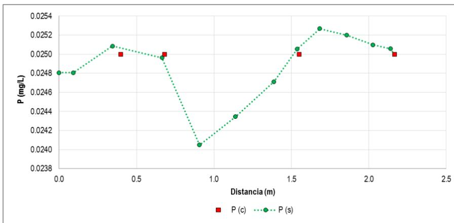
**Illustration 5-82.** Calibration results of organic phosphorus in the simulation section N ° 1.
