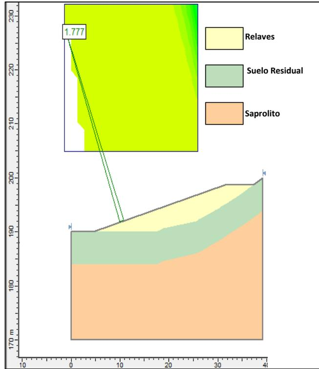
Illustration 5-12. Results of stability analysis under static conditions, Section B-B.
