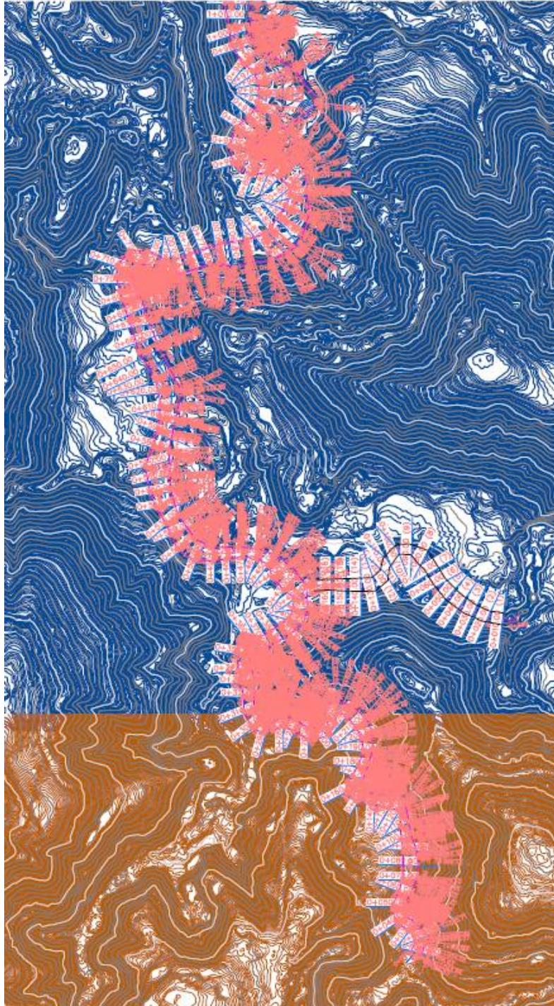
**Illustration 5-121.** Level curves extracted from the LIDAR image and location of the cross sections
