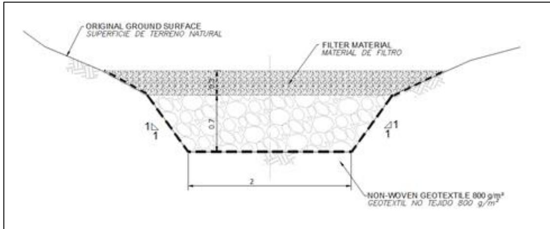
**Illustration 5-27.** Transverse section of the subdrainage in casting for tailings and / or sterile deposits.
