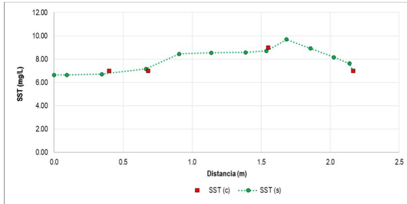
**Illustration 5-72.** Results calibration of the suspended solids in the simulation section N ° 1
