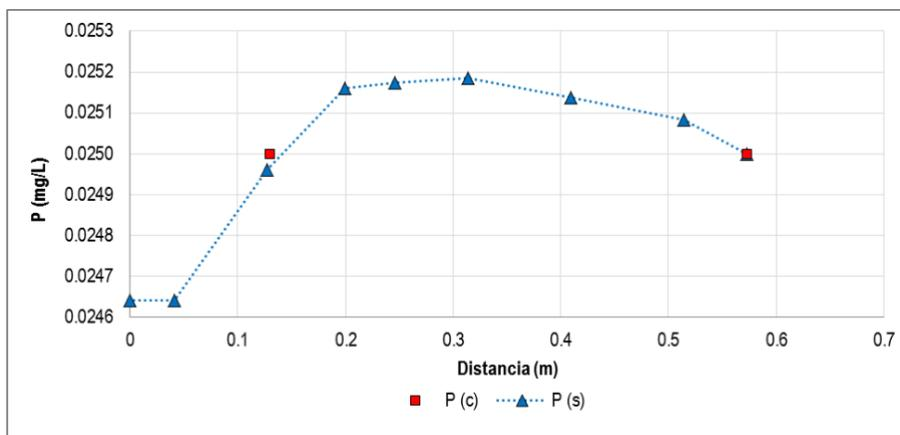
**Illustration 5-83.** Calibration results of organic phosphorus in simulation section No. 2.
