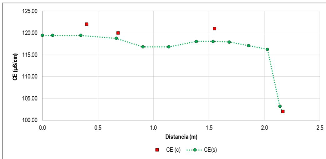
Illustration 5-70. Results calibration of the electrical conductivity in the simulation section N ° 1
