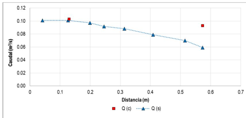
**Illustration 5-69.** Hydraulic calibration result of simulation section No. 2
