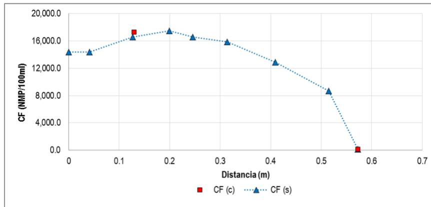
**Illustration 5-87.** Results calibration of fecal coliforms in the simulation section No. 2
