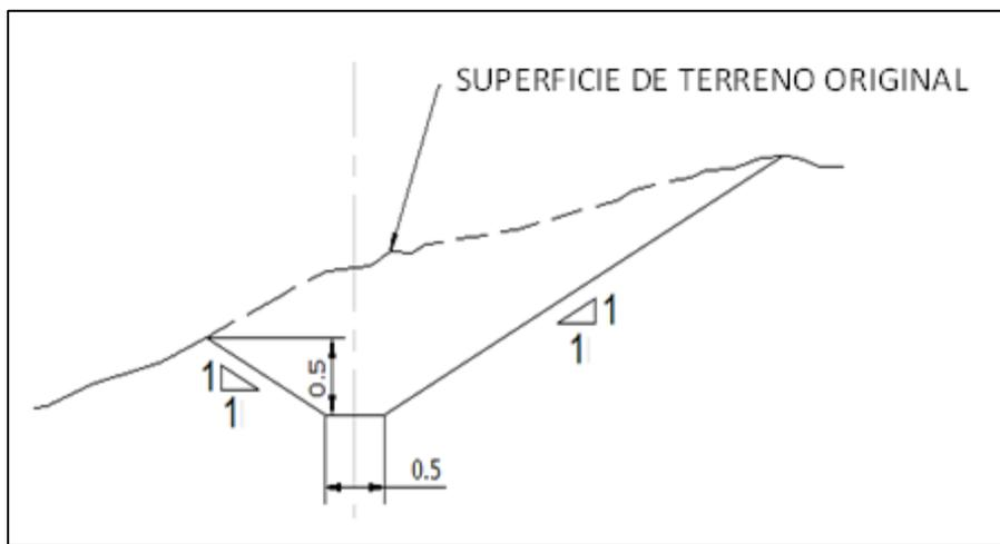
**Illustration 5-26.** Cross section for diversion channels.
