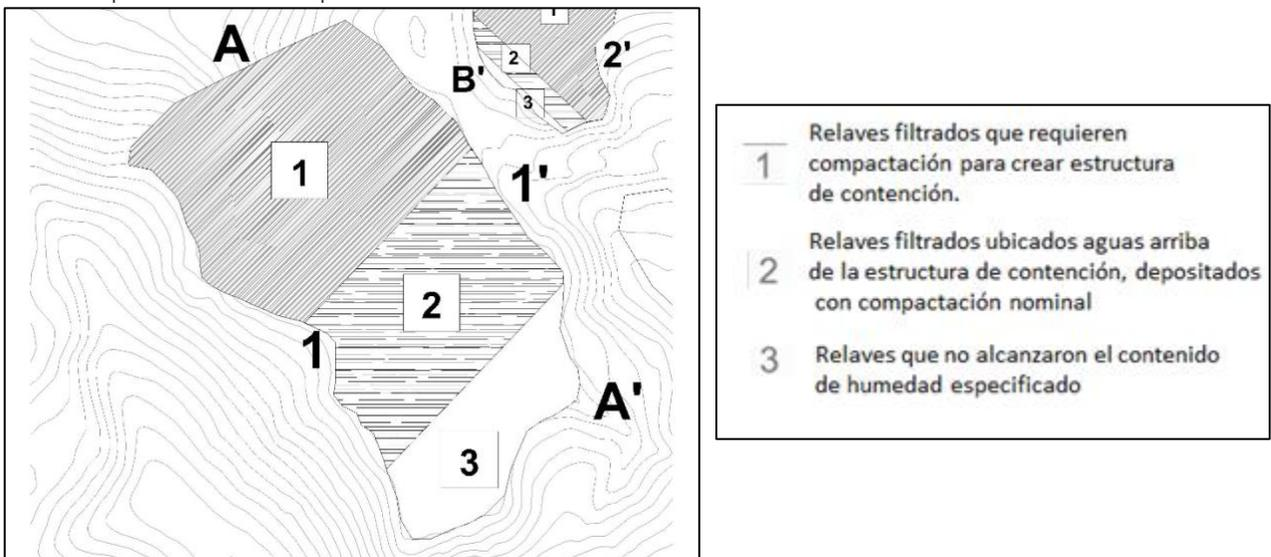
Illustration 5-4. Recommended compaction areas for tailings deposit No. 1.
