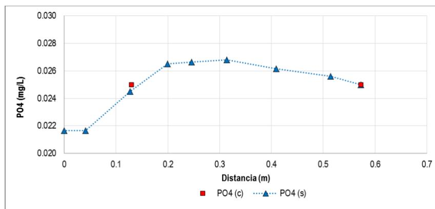
**Illustration 5-85.** Calibration results of inorganic phosphorus in simulation section No. 2
