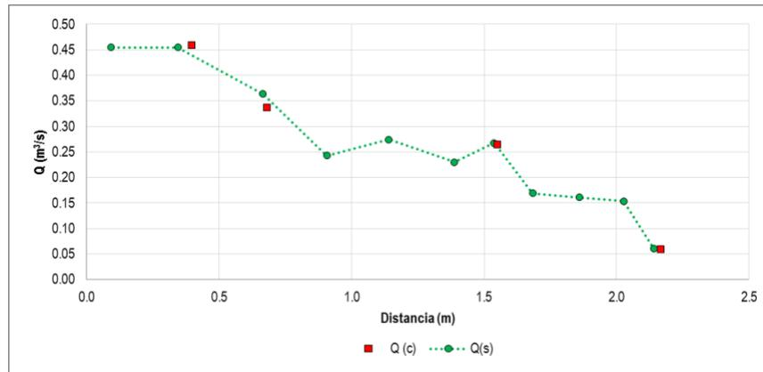
**Illustration 5-68.** Hydraulic calibration result of simulation section N ° 1
