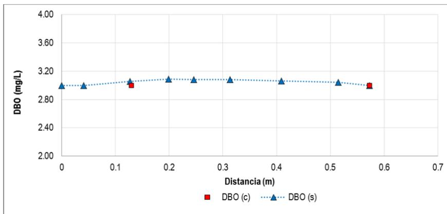
Illustration 5-77. Results calibration of the biochemical oxygen demand in the simulation section N ° 2
