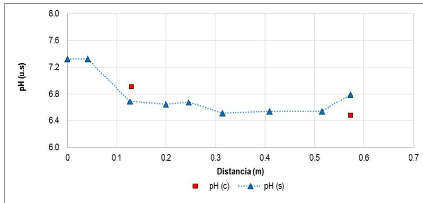
Illustration 5-93. Results calibration of the pH in the simulation section N ° 2
