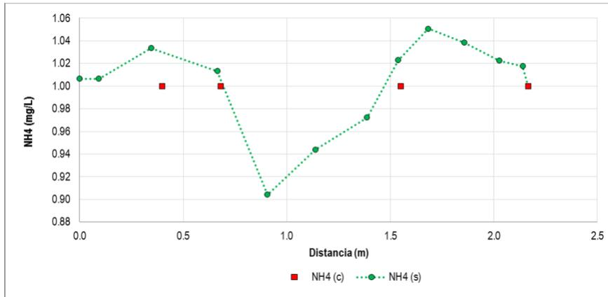
**Illustration 5-78.** Calibration results of ammonium in simulation section N ° 1
