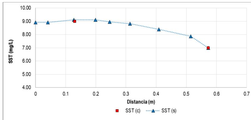
**Illustration 5-73.** Results calibration of the suspended solids in the simulation section N ° 2
