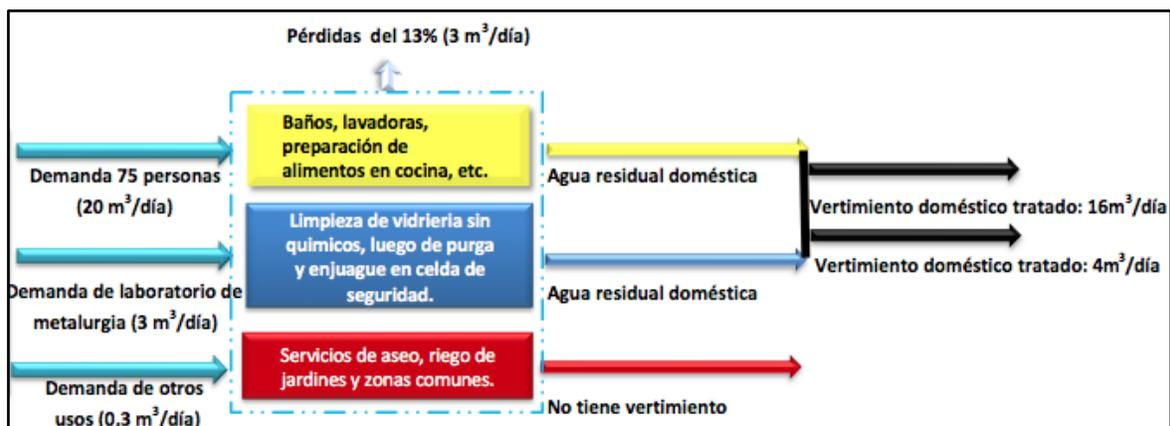
Illustration 5-20. Diagram of flow of supply and domestic discharges.
