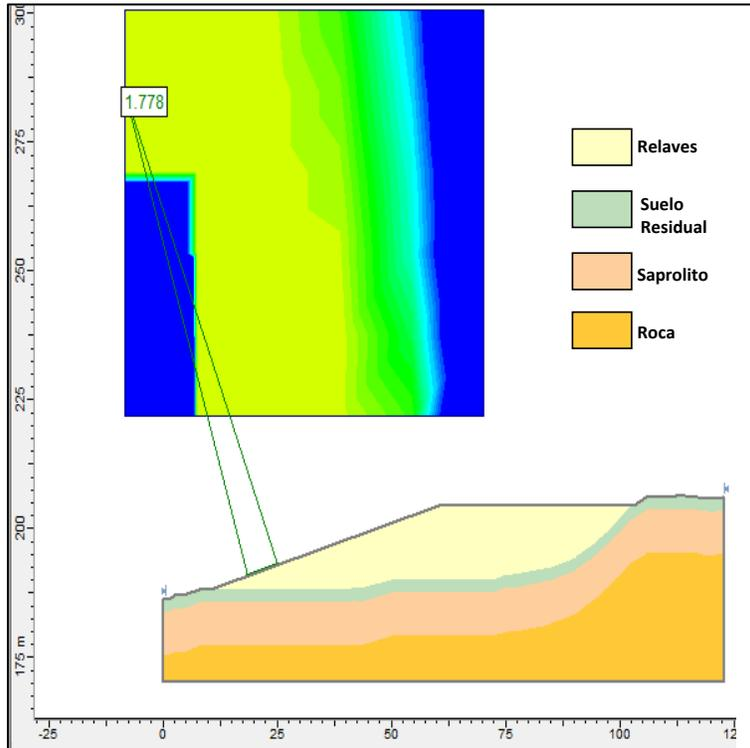
**Illustration 5-10.** Results of stability analysis under static conditions, Section A-A.
