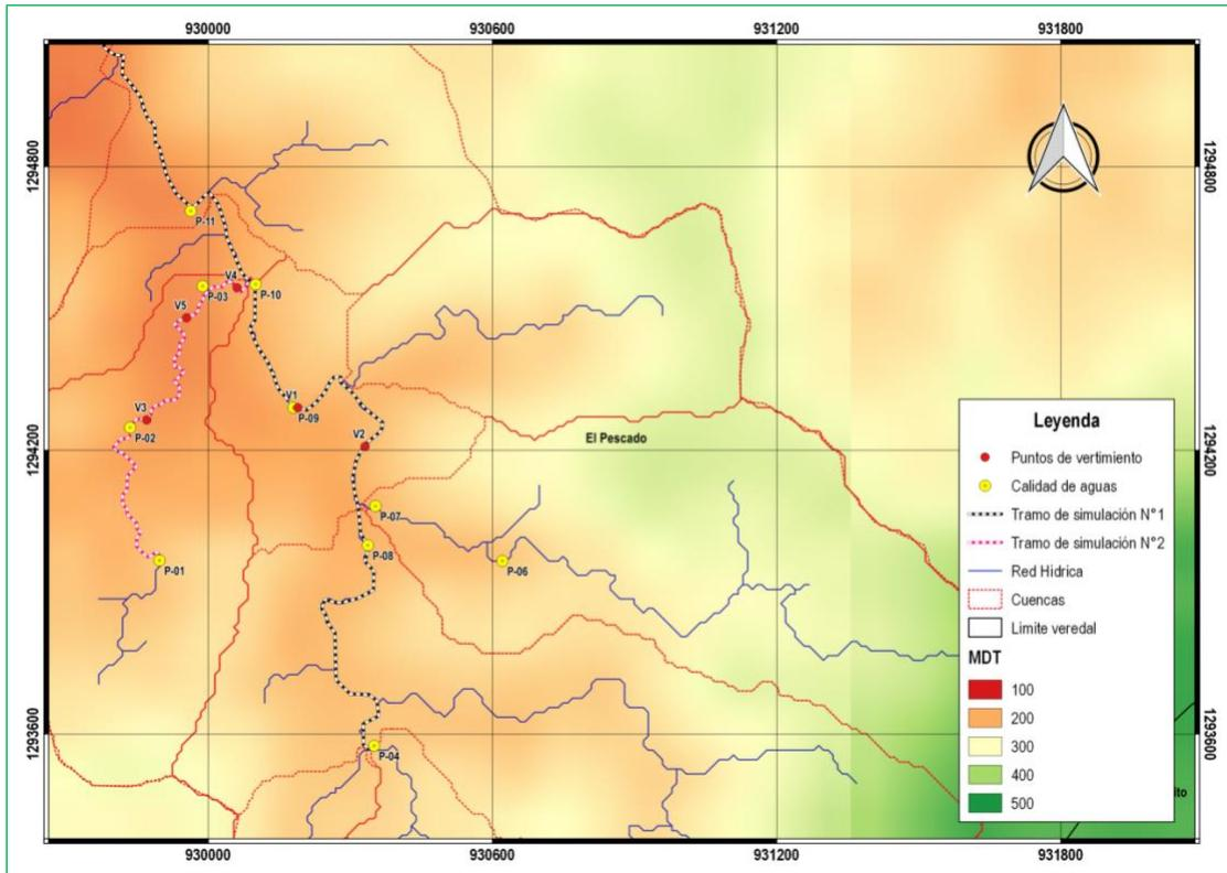
Illustration 5-35. Simulation stretches, water quality monitoring points and dumping points.
