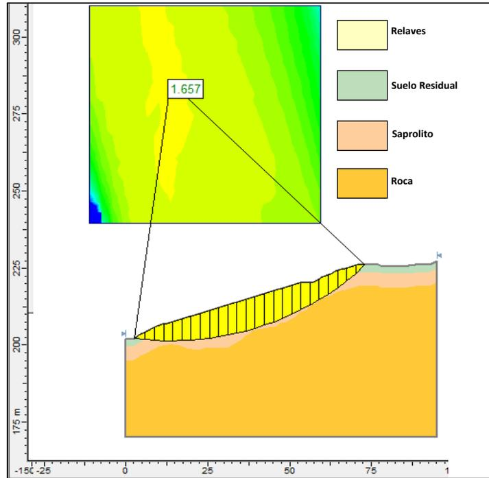
**Illustration 5-16.** Results of stability analysis under static conditions, Section D-D.
