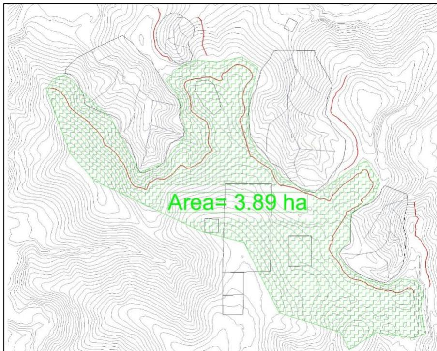
Illustration 5-25. Afferent area for the design of the channels for the tailings and/or sterile deposits.
