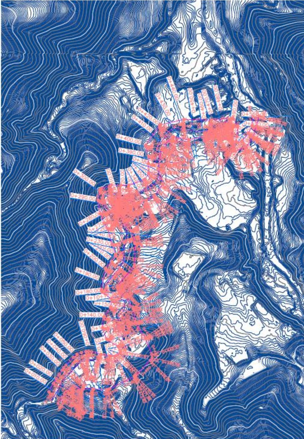
**Illustration 5-120.** Level curves extracted from the LIDAR image and location of the cross sections.
