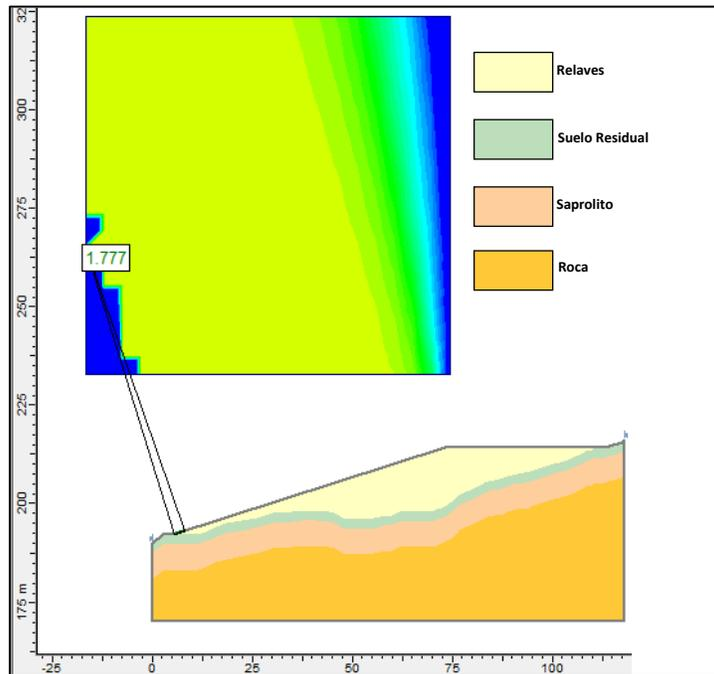
**Illustration 5-14.** Results of stability analysis under static conditions, Section C-C.
