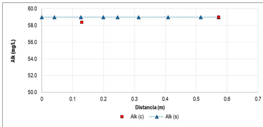
**Illustration 5-89.** Results calibration of the alkalinity in the simulation section N ° 2
