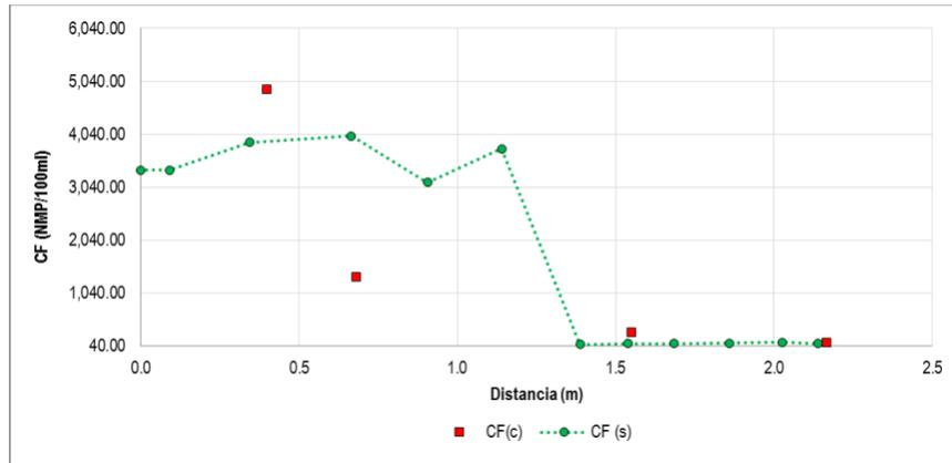
**Illustration 5-86.** Results calibration of fecal coliforms in the simulation section N ° 1
