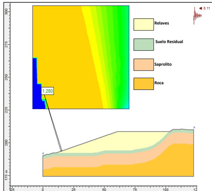
**Illustration 5-11.** Results of stability analysis under pseudo-static conditions, Section A-A.
