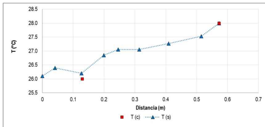
**Illustration 5-91.** Results calibration of the temperature in the simulation section N° 2
