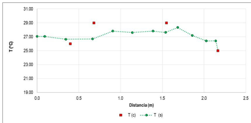
**Illustration 5-90.** Results calibration of the temperature in the simulation section N° 1
