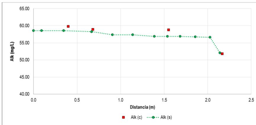
**Illustration 5-88.** Results calibration of the alkalinity in the simulation section N ° 1
