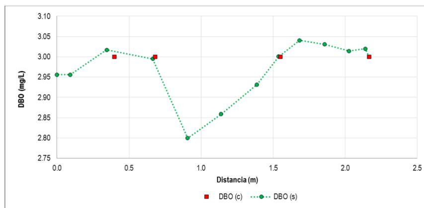
**Illustration 5-76.** Results calibration of the biochemical oxygen demand in the simulation section N ° 1
