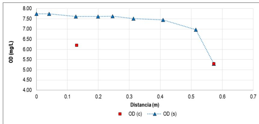
**Illustration 5-75.** Calibration results of dissolved oxygen in simulation section No. 2
