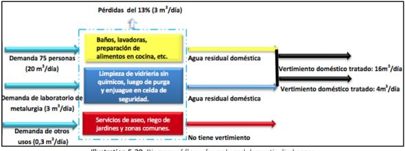
**Illustration 5-20.** Diagram of flow of supply and domestic discharges. *Source: INGEX, 2016.*
