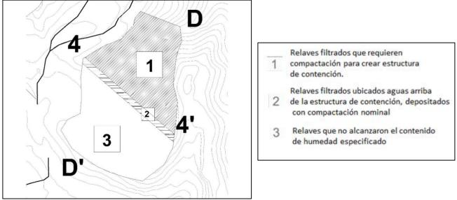
Illustration 5-7. Recommended compaction areas for tailings deposit No. 4. Source: INGEX, 2016
