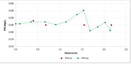
Illustration 5-84. Results calibration of inorganic phosphorus in the simulation section N ° 1 Source: INGEX, 2016
