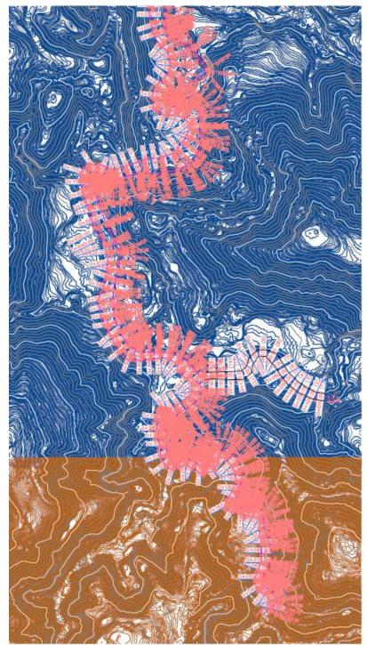
Illustration 5-121. Level curves extracted from the LIDAR image and location of the cross sections Source: INGEX, 2015
