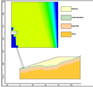
Illustration 5-14. Results of stability analysis under static conditions, Section C-C. Source: INGEX, 2016.
