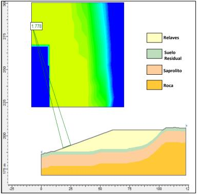
Illustration 5-10. Results of stability analysis under static conditions, Section A-A. *Source: INGEX, 2016.*
