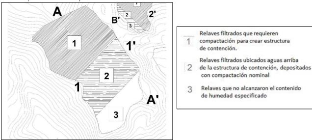
Illustration 5-4. Recommended compaction areas for tailings deposit No. 1. Source: INGEX, 2016
