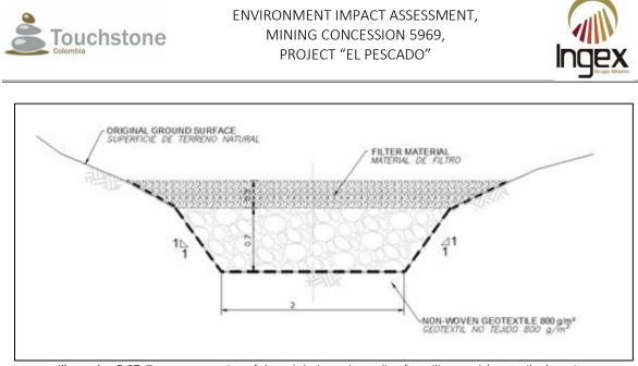
Illustration 5-27. Transverse section of the subdrainage in castling for tailings and / or sterile deposits. Source: INGEX, 2016
