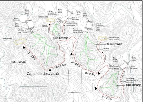
Illustration 5-24. Water management system for tailings and/or sterile deposits. Source: INGEX, 2016.
