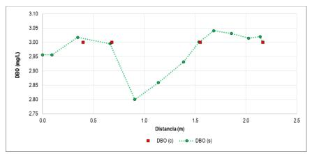
**Illustration 5-76.** Results calibration of the biochemical oxygen demand in the simulation section N ° 1 *Source: INGEX, 2016*
