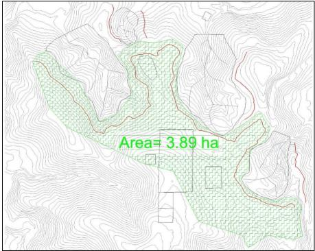
Illustration 5-25. Afferent area for the design of the channels for the tailings and/or sterile deposits. Source: INGEX, 2016.
