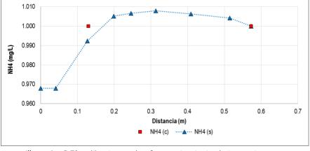
Illustration 5-79. Calibration results of ammonium in simulation section No. 2 Source: INGEX, 2016
