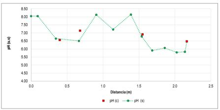
Illustration 5-92. Results calibration of the pH in the simulation section N ° 1 Source: INGEX, 2016
