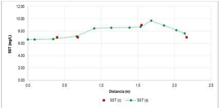
**Illustration 5-72.** Results calibration of the suspended solids in the simulation section N ° 1 Source: INGEX, 2016.
