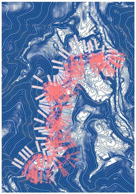
Illustration 5-120. Level curves extracted from the LIDAR image and location of the cross sections. Source: INGEX, 2016.
