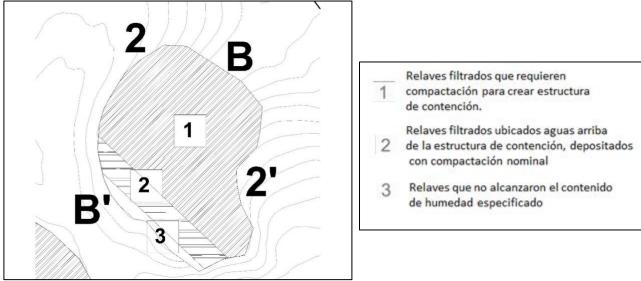
Illustration 5-5. Recommended compaction areas for tailings deposit No. 2. Source: INGEX, 2016
