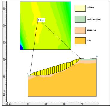
Illustration 5-16. Results of stability analysis under static conditions, Section D-D. Source: INGEX, 2016.
