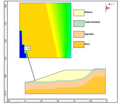
Illustration 5-11. Results of stability analysis under pseudo-static conditions, Section A-A. Source: INGEX, 2016.
