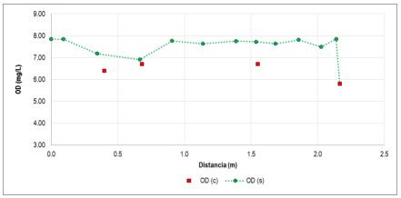
**Illustration 5-74.** Results calibration of the dissolved oxygen in the simulation section N ° 1 *Source: INGEX, 2014.*
