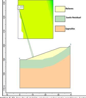
Illustration 5-12. Results of stability analysis under static conditions, Section B-B. Source: INGEX, 2016.
