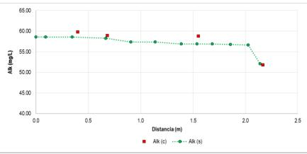
Illustration 5-88. Results calibration of the alkalinity in the simulation section N  $^\circ$  1  $_{Source:\ INGEX,\ 2016}$
