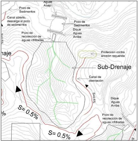
Illustration 5-30. General plant for water management wells for deposit No. 3. Source: INGEX, 2016.
