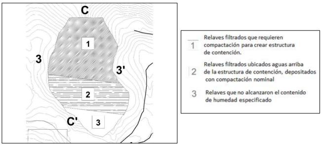
Illustration 5-6. Recommended compaction areas for tailings deposit No. 3. Source: INGEX, 2016
