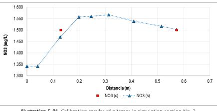
Illustration 5-81. Calibration results of nitrates in simulation section No. 2 Source: INGEX, 2016
