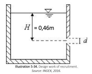
The design of this free-hole weir work determines the vertical location of the orifice with regarding the level of the sheet of water; by the Torricelli equation in terms of the flow, the cross-sectional area of the pipeline and gravity.
