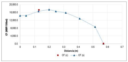
Illustration 5-87. Results calibration of fecal coliforms in the simulation section No. 2 Source: INGEX, 2016
