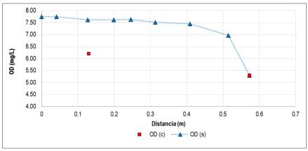
Illustration 5-75. Calibration results of dissolved oxygen in simulation section No. 2 Source: INGEX, 2016.
