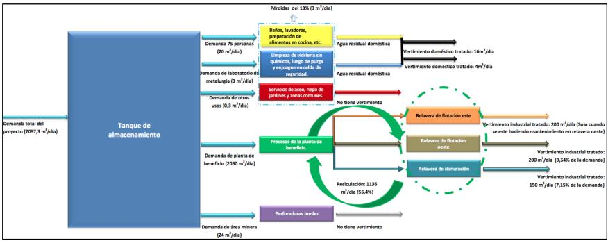
Illustration 5-19. Flow diagram of supply and dumping of the project.
