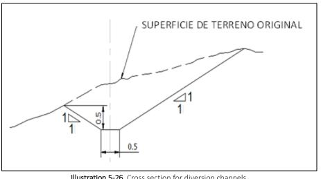
Illustration 5-26. Cross section for diversion channels. Source: INGEX, 2016
