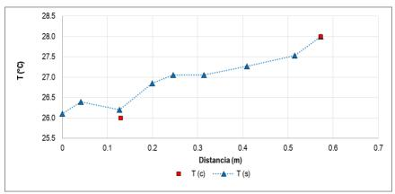
Illustration 5-91. Results calibration of the temperature in the simulation section N ° 2 Source: INGEX, 2016
