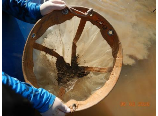
Figure 434 – The washing of the sediments on a sieve with an aperture of 250 µm.
