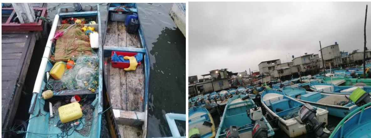
Photograph 16. Left: Boats that lack compartments to preserve fish and require short trips. Right: Fiberglass boats of greater length with cellar-type compartments, the most widely used vessel in the artisanal fishing subsector in the area of influence.
