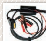
Senzor RPM inductiv (addon 007935900320) • 007935900345
