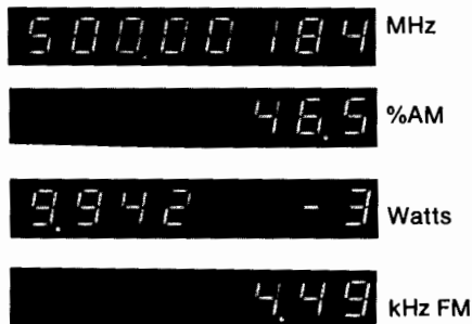
Modulation Analyzer displays of RF signal parameters.
