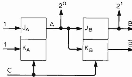
Fig. 3. Two-stage (scale-of-four) counter state diagram and codes (a) and circuit embodiment (b).
