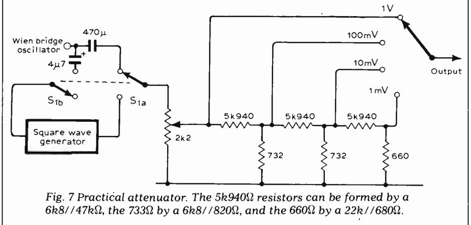
Fig. 7 Practical attenuator. The 5k940Ω resistors can be formed by a 6k8//47kΩ, the 733Ω by a 6k8//820Ω, and the 660Ω by a 22k//680Ω.
