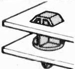
**P.C. BOARD STAND-OFFS** are quickly assembled, self-retaining panel supports for p.c. boards. Made from natural (off white) nylon and have good resistance to vibration. Suitable for panels up to 0.079" thickness. Stand-Offs accept a No. 4 self-tapping screw.
