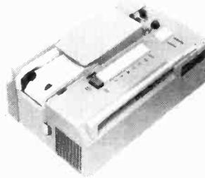
Polarized moving iron movements with syphon pens directly attached. Built-in solid state amplifier (one per channel) provides 8 calibrated sensitivity steps. Two marker pens are provided.
