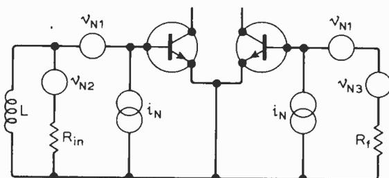
Fig. A4. Equivalent noise circuit of long-tailed pair stage.
