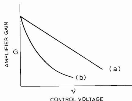
Fig. 3. Relationships of amplifier gain  $G$  versus control voltage  $v$ . Linear trace (a) will not provide a constant loop gain but exponential curve (b) produces a constant loop gain for all values of  $G$ .
