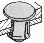
**LOKUT ANCHORS** are used to strengthen holes by providing additional screw thread engagement in materials where self-tapping screws would be unsatisfactory. Made from high strength nylon and used in insulation, and electrical chassis work. Easily fitted by hand.
