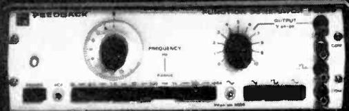
**2... 601 Function Generator. All the features of the 600 plus 0.001Hz to 1 MHz, 20V pk-pk output.**
