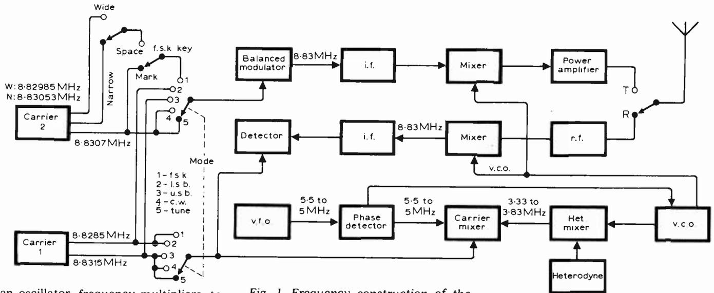
Fig. 1. Frequency construction of the Trio TS-820 h.f. transceiver. A phase lock loop is used for frequency derivation and the circuit employs a double carrier system to allow sideband switching without re-calibration. See text.
