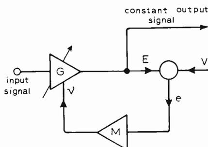
Fig. 2. Negative feedback arrangement used in automatic gain control systems.
