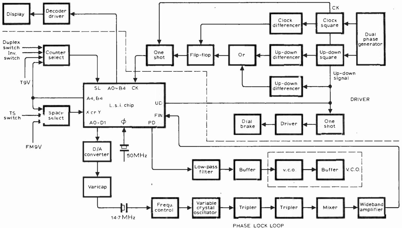
Fig. 4. Block diagram for the first mixer oscillator used in the Icom IC-211E and IC-245E transceivers. This system uses a m.o.s. l.s.i. chip to provide v.f.o. tuning coupled with p.l.l. digital-synthesized circuitry. See text.
