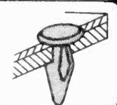
**PLASTIC HOLE PLUGS** are quick, inexpensive means of plugging unwanted holes. Hole Plugs keep out dust, dirt and moisture. Attractively shaped heads give a neat finish. The snap action grip of the Hole Plug makes a vibration resistant seal. Hole Plugs are made from nylon and are non-corrosive.
