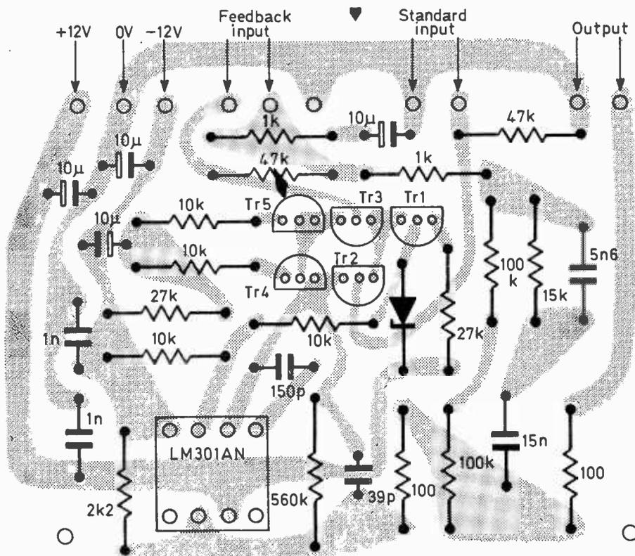
The maximum output signal amplitude before clipping is 5.6V r.m.s. which gives a 35dB overload capability referred to 100mV.
