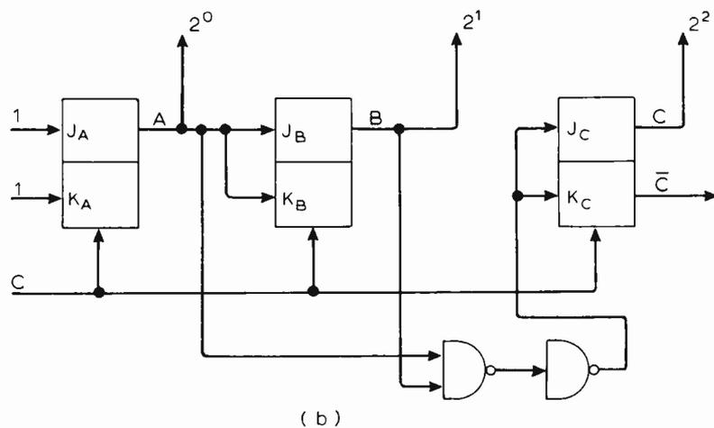
Fig. 4. State diagram (a) and circuit (b) of three-stage (scale-of-eight) counter.
