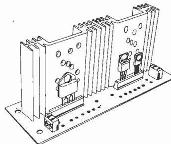
Power semiconductor devices can't easily be used on breadboards. Now Ramp's Power Board solves the problem. T03 and T066 metal devices, and T03P, T066P, T0127 and T0220 plastic devices fit rapidly onto two ten watt heatsinks, and connect simply into the breadboard without soldering. T092 devices can be fitted for thermal stabilisation.
