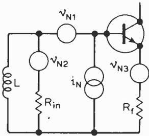
where  $v_{N1}$  is the equivalent noise voltage generator of the transistor,  $v_{N2}$  the equivalent noise voltage generator of the input resistance  $R_{in}$ ,  $v_{N3}$  the equivalent noise voltage generator of the equivalent feedback network resistance  $R_f$ ,  $i_N$  the equivalent noise current generator of the transistor, and  $L$  the inductance of the magnetic cartridge, assumed purely inductive.
