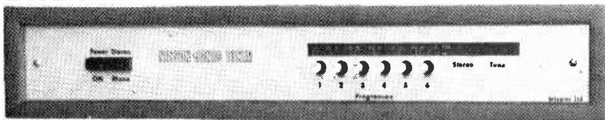
**Brief Spec.** Tuning range 88—104MHz. 20dB mono quieting @ 0.75 $\mu$ V. Image rejection — 70dB. IF rejection — 85dB. THD typically 0.4%. IC stabilized PSU and LED tuning indicators. Push-button tuning and AFC unit. Choice of either mono or stereo with a choice of stereo decoders.
