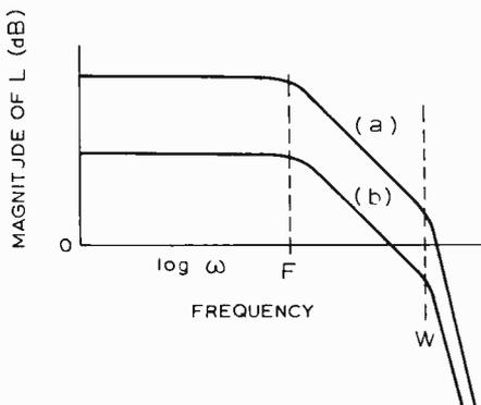
Fig.5. Graphs illustrating that variations in zero-frequency loop gain can cause instability. Curve (a) crosses the 0dB point (unity-loop gain) with a slope of 12dB per octave corresponding to a loop phase shift of 180 degrees. Curve (b) is stable because the loop phase shift is 90 degrees at unity loop gain.
