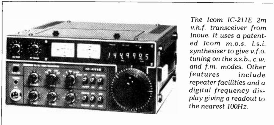
The Icom IC-211E 2m v.h.f. transceiver from Inoue. It uses a patented Icom m.o.s. l.s.i. synthesiser to give v.f.o. tuning on the s.s.b., c.w. and f.m. modes. Other features include repeater facilities and a digital frequency display giving a readout to the nearest 100Hz.
