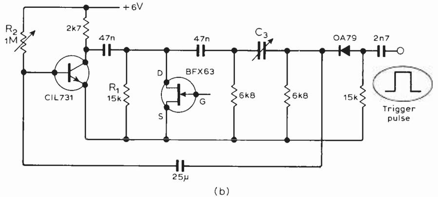
sections of the oscillator. By applying a positive trigger pulse at the transistor base, the circuit starts to oscillate. Resistor  $R_2$  is adjusted so that the oscillations cannot be sustained and hence decay gradually. One method of obtaining drum sounds of different tonal quality is to vary  $C_3$  which changes both the frequency and the envelope of the waveform. Quality and
