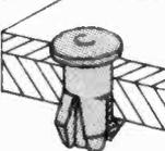
**DRIVE FASTENERS** hold two or more panels together. Easily fixed, normally by thumb pressure. No special tools required. Boat-shaped DRIVE Fasteners are for panels of thin and medium thickness and are removable. Ribbed Drive Fasteners are used in blind holes where hole length exceeds length of shank.
