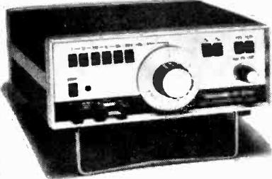
G432 is a source of sine, square and triangle signals, 1Hz to 1.1MHz. 5V from 50Ω, via attenuator.
