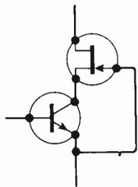
Fig. 3. Bipolar f.e.t. cascode arrangement.
