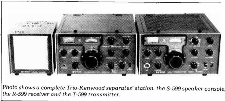
Photo shows a complete Trio-Kenwood separates' station, the S-599 speaker console, the R-599 receiver and the T-599 transmitter.
