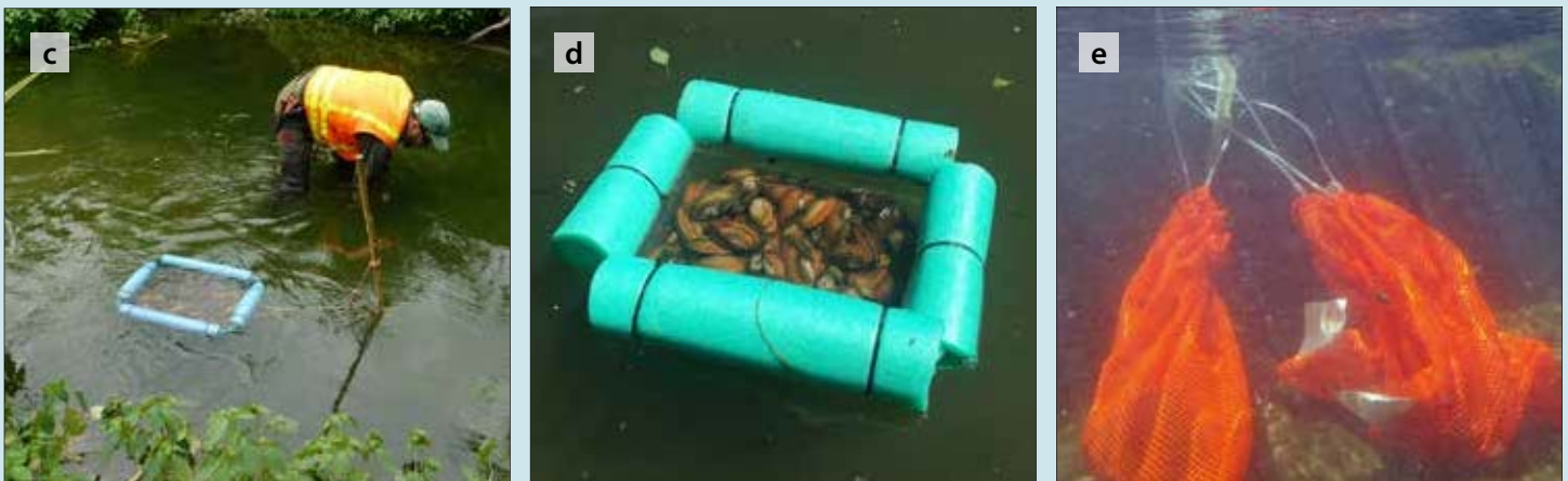
Figure A3.3: c–d: This "mussel raft" was designed using a plastic box with holes punched through to allow water to flow over mussels. The pool noodles ensure that the device floats, enabling mussels to stay cool and submerged if they are collected for species identification or density estimates (design and construction of mussel raft by Patrick Norton). e: Mesh bags are also commonly used to temporarily hold mussels.
