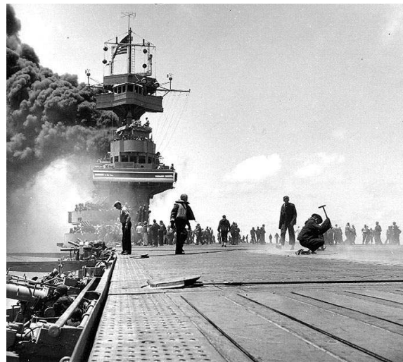
Photo # 80-G-312018 On board USS Yorktown after she was hit by dive bombers Scene on board USS Yorktown (CV-5), shortly after she was hit by three Japanese bombs on 4 June 1942. Dense smoke is from fires in her uptakes, caused by a bomb that punctured them and knocked out her boilers.
