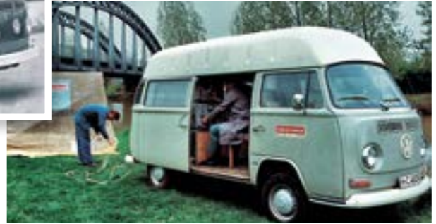
The high-roof Transporter T2 featured a composite roof and sliding side door.
