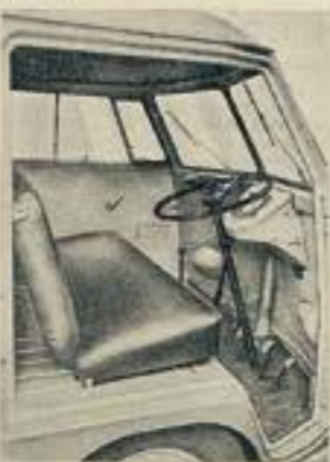
The wide forward-hinged door provides easy access to the cab, which has a bench-type seat. The heater duct is seen attached to the front panel.
