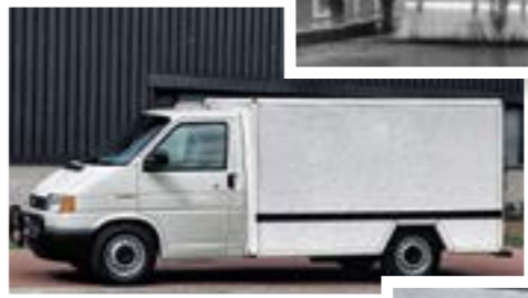
A T4 chassis cab equipped with a low-roof box body. A similar body could be refrigerated.
