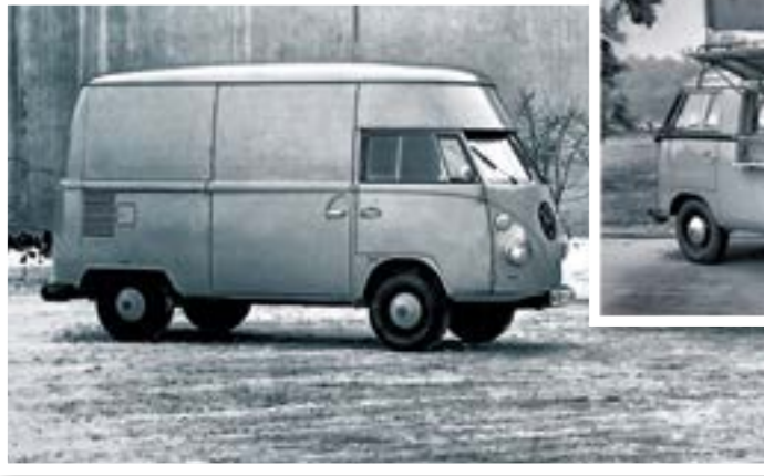
This T1 high-roof factory prototype was produced for the Bundespost and features a sliding door.
