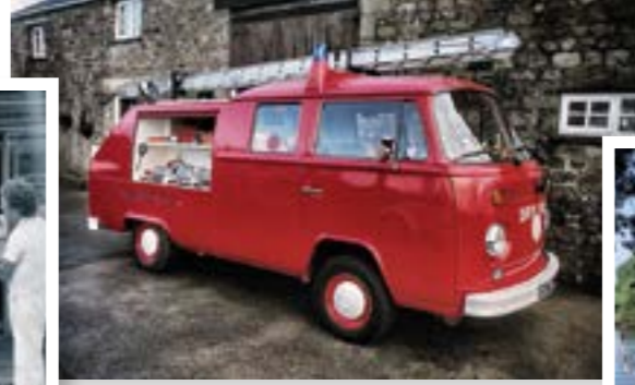
UK fire truck conversion built on a Pick-up chassis by Brainbridge Fire and Security.
