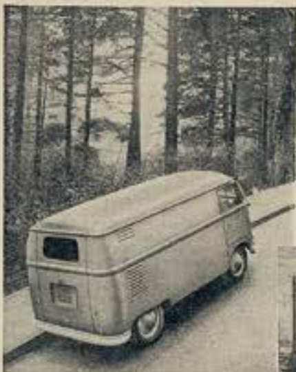
(Above) Stop-start tests were accomplished on a 1 in 4½ gradient when carrying part load. The Volkswagen has a smart appearance with modern styling. (Right) The van is seen here approaching Ludgate Circus, with Holborn Viaduct in the background, during its trials in London traffic.
