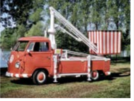
SO 10 was a hydraulic lifting platform model, commonly known as a 'Cherry Picker'.
