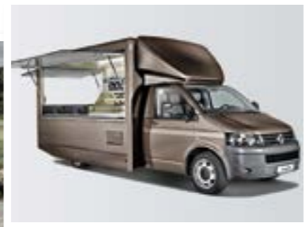
This mobile shop is built on a T5 chassis cab and features a high roof and hinged side panels that double up as shelter for waiting customers.
