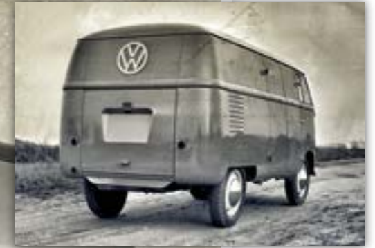
Rear view of an early vehicle (pre November 1950), identifiable by the badge. Early vehicles did not have rear windows or rear bumpers.
