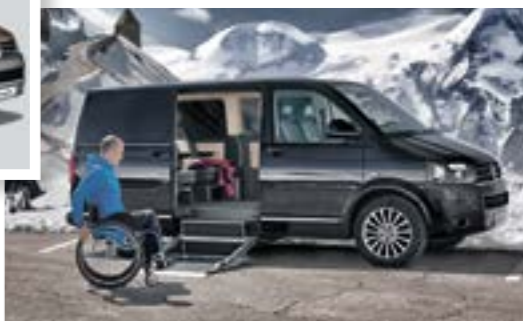
A wheelchair-accessible T5 Business with pavement access via an under-floor mounted electric lift.
