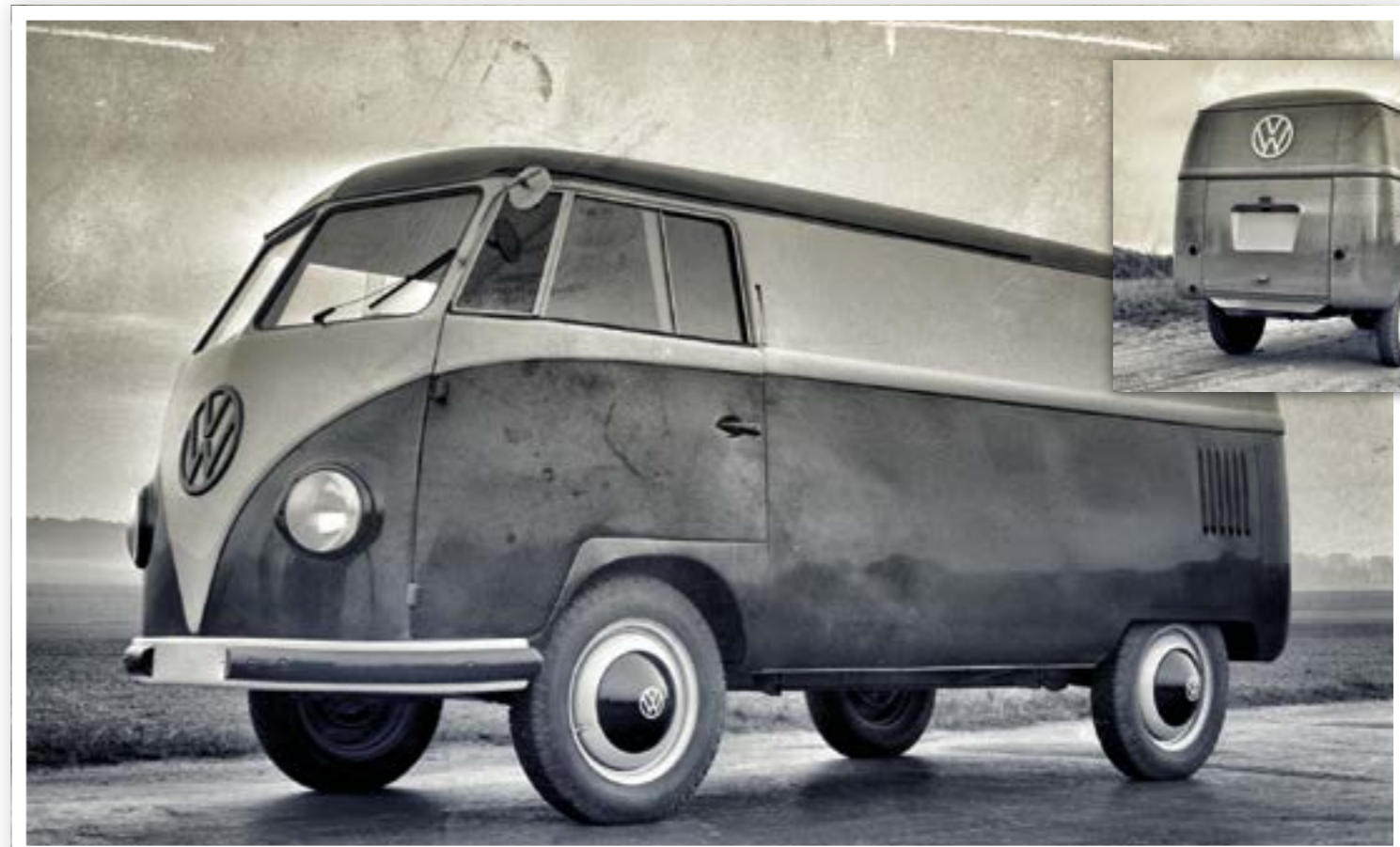
An early prototype finished in striking two-tone paintwork. Note the vertical rear cooling vents.
