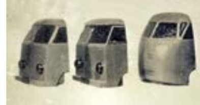
Original blueprints for project EA-7. Wind tunnel testing which improved the drag coefficient to an impressive 0.4.
