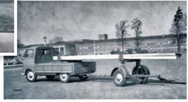
A novel use for a pick-up bed. Equipped with a swivelling attachment, long loads could be towed in combination with a lightweight trailer.
