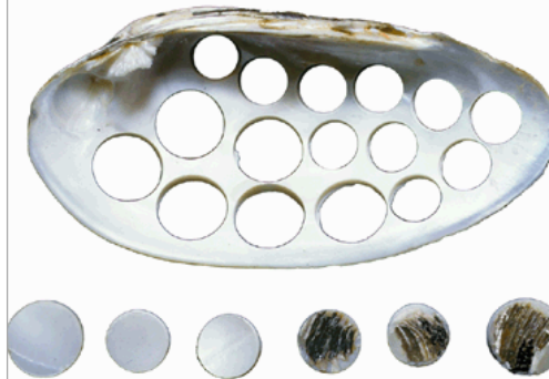
Button shell (Yellow sandshell; Lampsilis teres ) and button blanks
