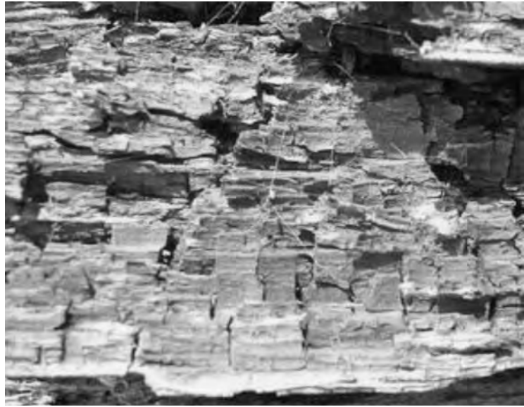
Fig. 11.19 Part of a pine stump showing the characteristic brick-like decay by brown-rot fungi.
