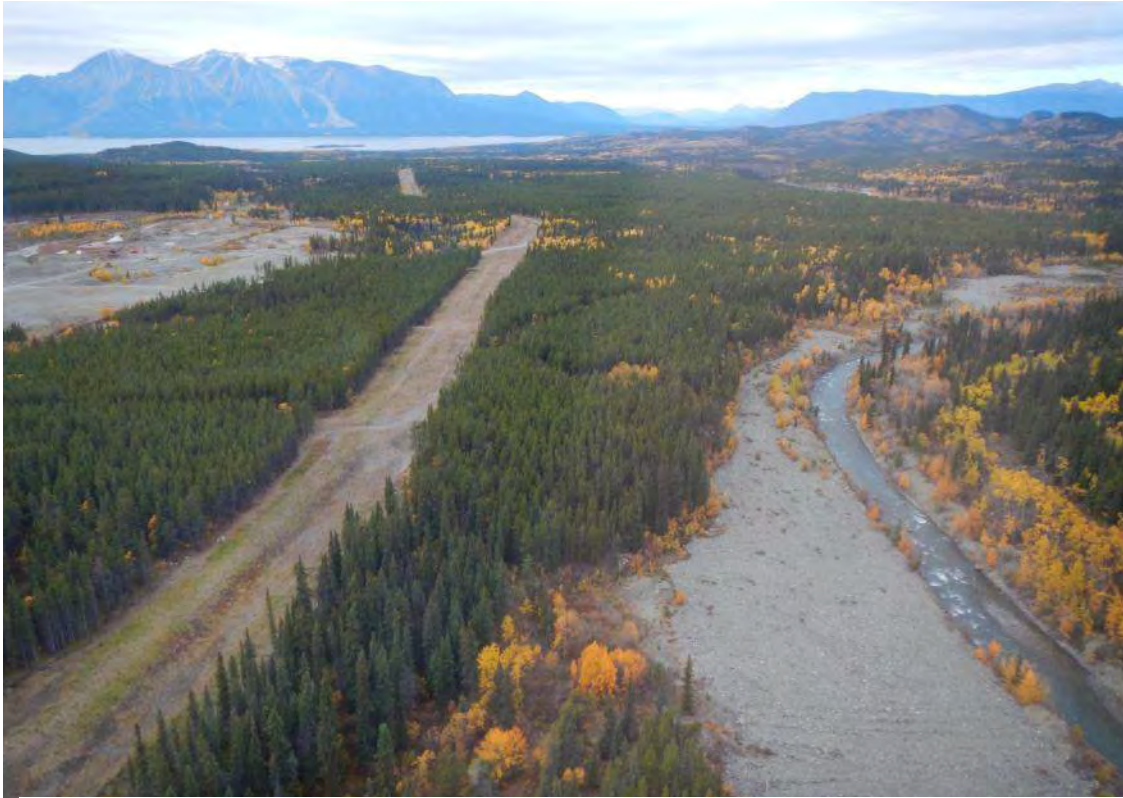
Photo 4. Existing penstock right of way, looking downstream (west). Penstock in on the left, service road on the right side of the clearing.
