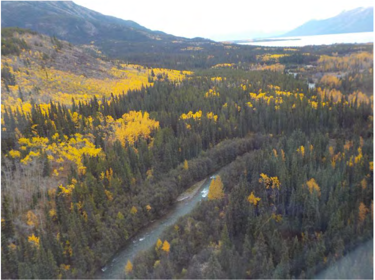
Photo 3: Proposed lower penstock alignment on south side of Pine Creek (left side), looking downstream. Note the low saddle between hill in mid-ground and mountain side on left side of photo.
