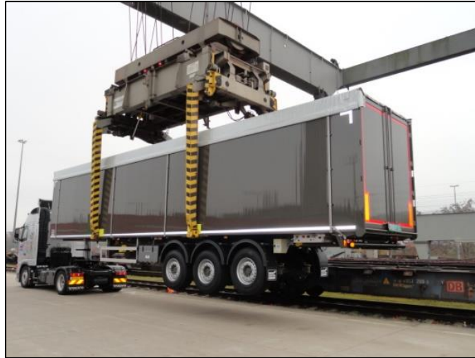
Figure 1: RMG (Rubber mounted gantry crane)
