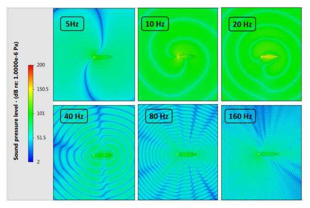
Figure 7. Sound propagation pattern at various frequencies using BEM for propeller noise including scattering effect
