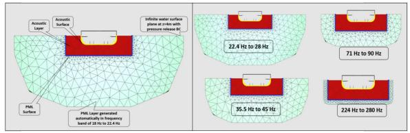
Figure 2(a) Left: PML model for Main Engine Room; Figure 2(b) Right: Adaptive PML generated for various frequency bands
