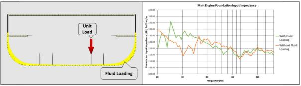
Figure 4(a) Left: ME room section; Figure 4(b) Right: ME foundation input impedance
