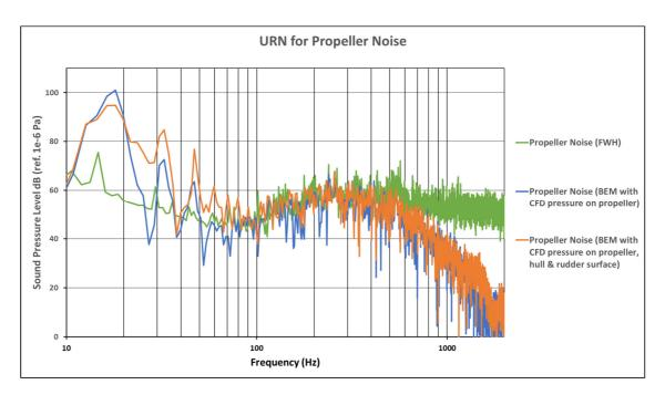
Figure 8 URN from propeller as a noise source for various numerical models
