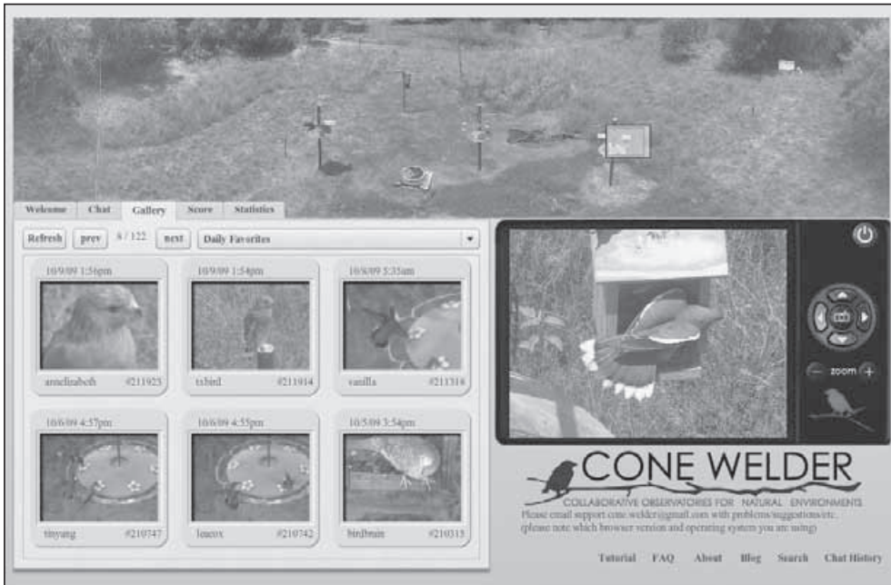
FIG. 2. Interface of the website ( http://cone.berkeley.edu ) for the collaborative telerobotic wildlife camera system, CONE Welder. The top panorama illustrates the camera field of view, which allows users to draw rectangles to control the camera. The camera window on the right side of the frame shows the live view. Each user can capture a picture by clicking on the camera button to the right of the live view. The image is then stored and displayed in the list at the left side of the live view, where users can enter their comments to annotate the image or comment on photos taken. Each user logs on to the system to draw rectangles on the panorama to indicate where they want the camera to observe. Details regarding camera operation can be found in Song (2009).
