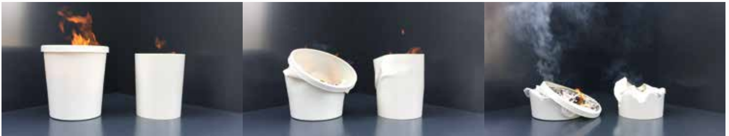
Standardpapierkorb vs. Sicherheitspapierkorb - standard waste bin vs. safety waste bin
