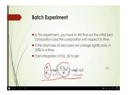
Now as per batch experiment, this experiment you have to first find out the initial bed composition and the composition with respect to time. Now, if the total mass of bed does not change significantly; that means, less than it is 20 percent in a time then integration of the equation 4 will give you that W i by W i0 that will be is equal to exponent of; that means, here minus k i star into a bed into t by W and; that means, your exponent of minus k i it.
