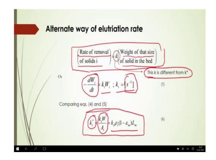
Now is there any other alternative way or not that there is one alternate way of elutriation rate that can be calculated, now if we represent this rate of removal of the solid of class i which is proportional to the weight of that size i of the solids in the bed, then what should be the proportionality constant that will be is k. So, this k is different from here k star.
