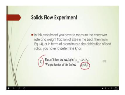
So, solid flow experiment as per solid flow experiment, you will see that you have to measure, the carry over rate and the weight fraction of the size in on the bed and then
