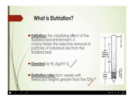
Which is exactly the unit for that solid flux here; W s unit is the; that means, kg per meter square second. And this elutriation rates from the vessel with freeboard height is greater than the TDH that will be should be remember.
