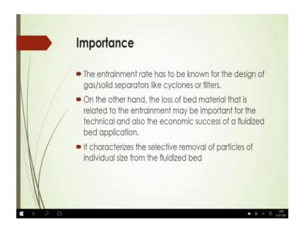
Now, what is the importance that for which you have to know that elutriation characteristics in the fluidized bed. Now you know that entrainment rate that has to be known for the design of gas solid separators like cyclones or filters, in the same way elutriation is also important because this give you the classification of the solid particles
