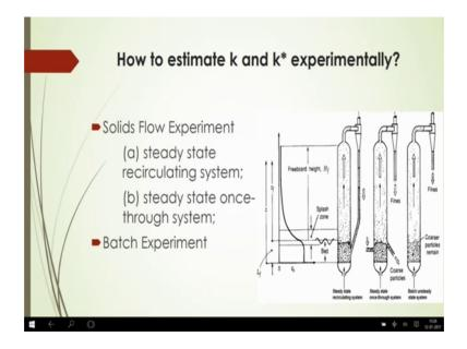
Now how to estimate k and k star experimentally? Now, solids flow experiments here you will see that one is steady state operation and steady state re circulating system and there will be a steady state once through system and another important experiment that as experiment. You can estimate this, this elutriation rate by this two types of a experiment there.
