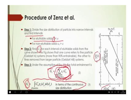
Now, Zenz et al model, as per that Zenz et al model you will get the different step to calculate that elutriation rate here. Now as a step 1, you can say that this distribution of the particle that will actually role enough there. So, you have to divide the size distribution of the particle into narrow intervals and then you have to find the intervals in such a way that, for elutriate for elutriable solids; that means, U f is less than u; that means, here or Ut here.
