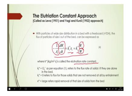
The elutriation constant approach here, it is called something is a Leva 1951 and Yagi and Kunli approach also. So, now, with particles of wide size distribution in a bed with a freeboard, which transport disengagement height is actually less than these a freeboard. The flux of particles of size i out of the bed can be expressed as by equation 4 here.
