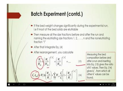
Now, if the bed weight changes significantly during the experimental run that is if most of the bed solids are elutriable. Then measure all the size fractions before and after the run. And rooming sorry and naming the elutriating size fractions 1, 2, to n and the nonelutriating fraction of i.
