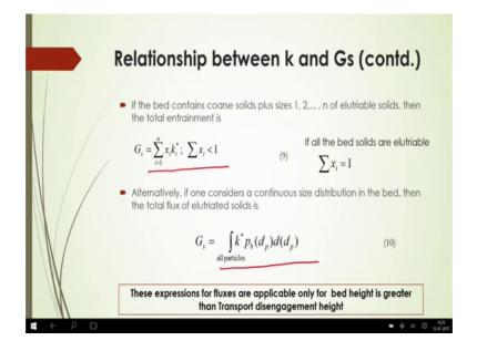
Now, here if the bed contains coarse solids plus sizes like 1, 2, 3 dot dot dot n; that means, n different size of a of solids which are elutriable and then, the total entrainment will be is equal to G s that will be is equal to their summation of i is equal to i to n, x i into k i star; that means, you have for all solid are classified a particles are there you have to sum up all those things.
