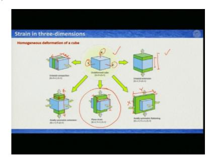
This diagram presents, this is the unit cube highlighted by a circle where X is vertical, Y and Z are oriented horizontally, this is un-deformed cube therefore XYZ equal to 1, now one can deform this cube in many different ways, but here what is shown by these five illustrations at these five sides, these are the some sort of end members of the deformation in three dimensions.
