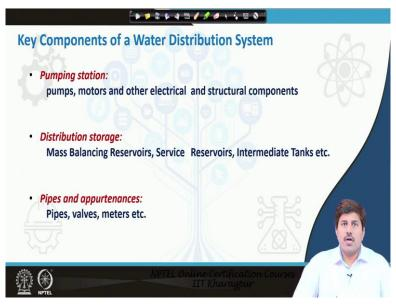
Now a typical water distribution system has 3 major components or three key components there is a pumping station which includes pump, motor or other electrical and structural components. There is a distribution storage which includes mass balancing reservoir or service reservoirs or at times intermediate tanks and then there are pipes walls meters those kind of facets which are there in the distribution network.
