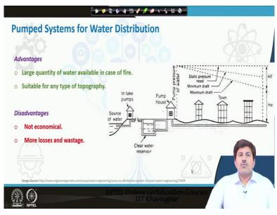
So the advantage include that large quantity of water is available in case of fire or in case of any emergency and second thing it can be suitable for any type of topography. Because we are not relying on the gravitational forces available for supply of water. We are providing additional forces through pump so we can use it for any kind of topography. The disadvantages include that it is not economical and there are going to be more losses and wastage because we are pumping the water altogether.
