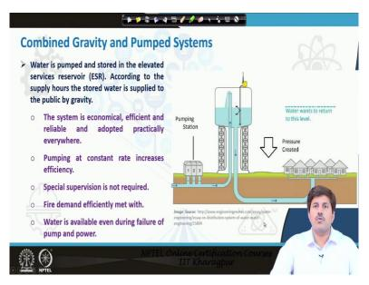
However generally none of these 2 systems are very common the one that most common is the combined gravity and pumped system or dual system where water is pumped and stored at an elevated service reservoir and then which is basically a kind of place where we do all the; we store water for supply purpose and then from there we supply water at the rate desired and in case of emergencies we can use these storage for supplying additional water as well.
