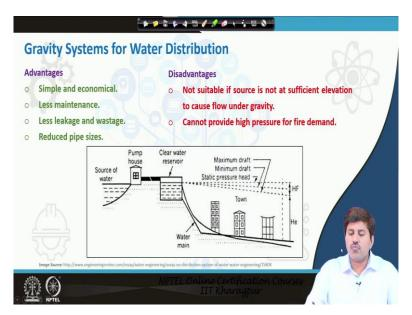
Also water wastage and leakages are minimized in such system because we are not providing any additional pressure so the advantage include that the system is simple and economical it requires less maintenance there is less leakage and wastage. There are relatively reduced pipe sizes for the flow. The disadvantage is; it is not suitable if the sufficient head is not available at the source. So, that is the very basic criteria that source should have the sufficient head.
