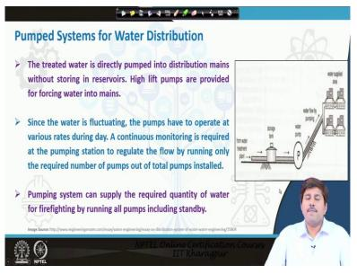
Then there are a pump system for water distribution these are basically the directly pumped into the distribution means without any like other storage reservoir or we may provide a storage reservoir we may need say MBR or mass balancing reservoir at times but otherwise it may directly be basically sending to the elevated storage reservoirs. So, here the water might be basically fluctuating so pump have to operate at various rates during the day period.
