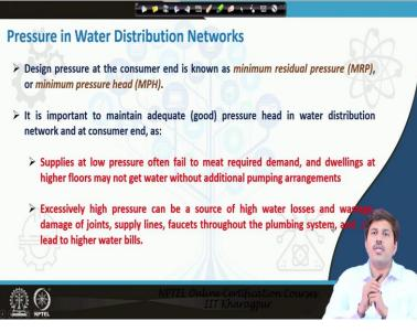
So, pressure head maintenance in the water distribution network is a very high importance we must share like we must ensure while designing a system that the pressure at the consumer end is adequate and which is typically liked for design purpose it is known as minimum residual pressure which is MRP or minimum pressure head MPH. So, we should ensure that these requirements are met. It is important to kind of maintain adequate or good pressure head in distribution network.
