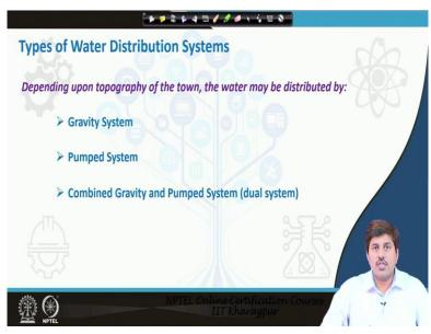
Now there are 3 types of water distribution networks there have a gravity system there is pumped system and there is a combined gravity and pump system which is known as dual system.
