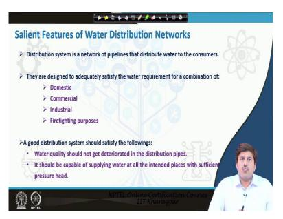
Now a typical water distribution network is a connection or network of pipelines that distribute water to the end consumers and they are designed to kind of satisfy the water requirements for domestic purpose for commercial purpose for industrial purpose for fire fighting purpose and often a combination of these. Industrial supply maybe separate at times but generally domestic commercial and fire fighting applications are met with this single network.
