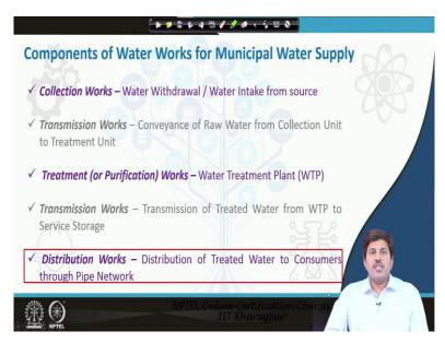
To begin with if you like again revise what we discussed earlier that what are the different components of a waterworks for municipal water supply? So, we started with the collection works where we basically collect water or withdraw water through water intake from the source. Then there is a transmission works which is responsible for conveyance of raw water from collection unit to the treatment unit that also we discussed.
