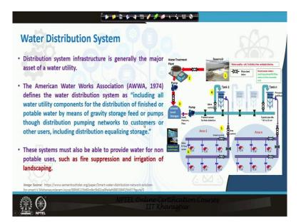
So, essentially if you see we get the water and then through if this is basically the point of purification or treatment facility. So, from treatment facility we put the water again the water through distribution mains or treated water mains to a service storage or storage it is a wire label and from there we basically put it to a distribution system. So, water distribution system is basically interest is one of the major asset of a water utility in terms of infrastructure.
