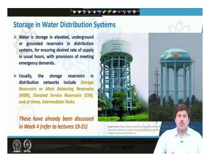
So, if these in these 3 network in these 3 basic requirements the storage in the water distribution system is one of the key kind of component of a water distribution system. So, water is typically stored in the elevated underground or ground reservoirs depending on the topography available. Many times just underground reservoirs are used many times the like partially underground and partially surface or partially grounded reservoirs are used and many times elevated reservoirs are used.
