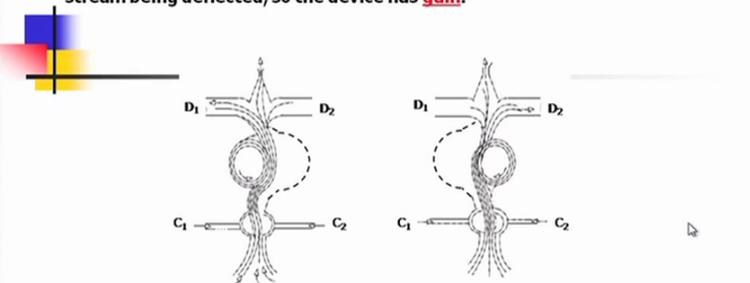
Fig.- 7.27-1 Fluidic amplifier, showing flow in both states. Ref: U.S. Patent #4,000,757.
