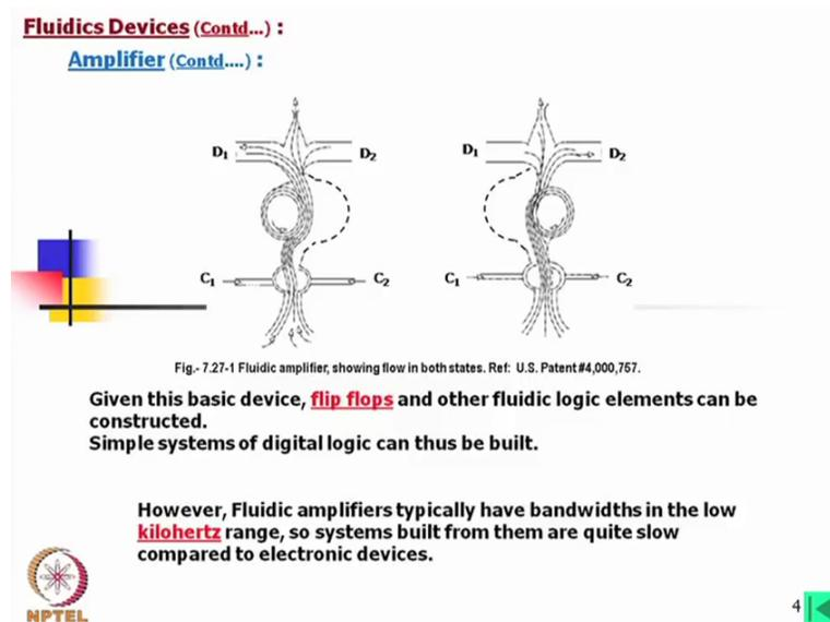
Now with this basic device, the flip-flops and other fluidic logic elements also can be constructed, basic principle remains same. Simple systems of digital logic can thus be built, this means we have already learned about the digital logic, now with this we can make the device which are called Gates different types of Gates and with these gates we can build the logic and we can construct also physical circuits.
