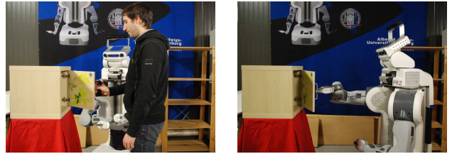
Fig. 1: Learning from human demonstrations: The robot observes the human demonstrating a task, adapts this to its own capabilities and executes the task on its own.
