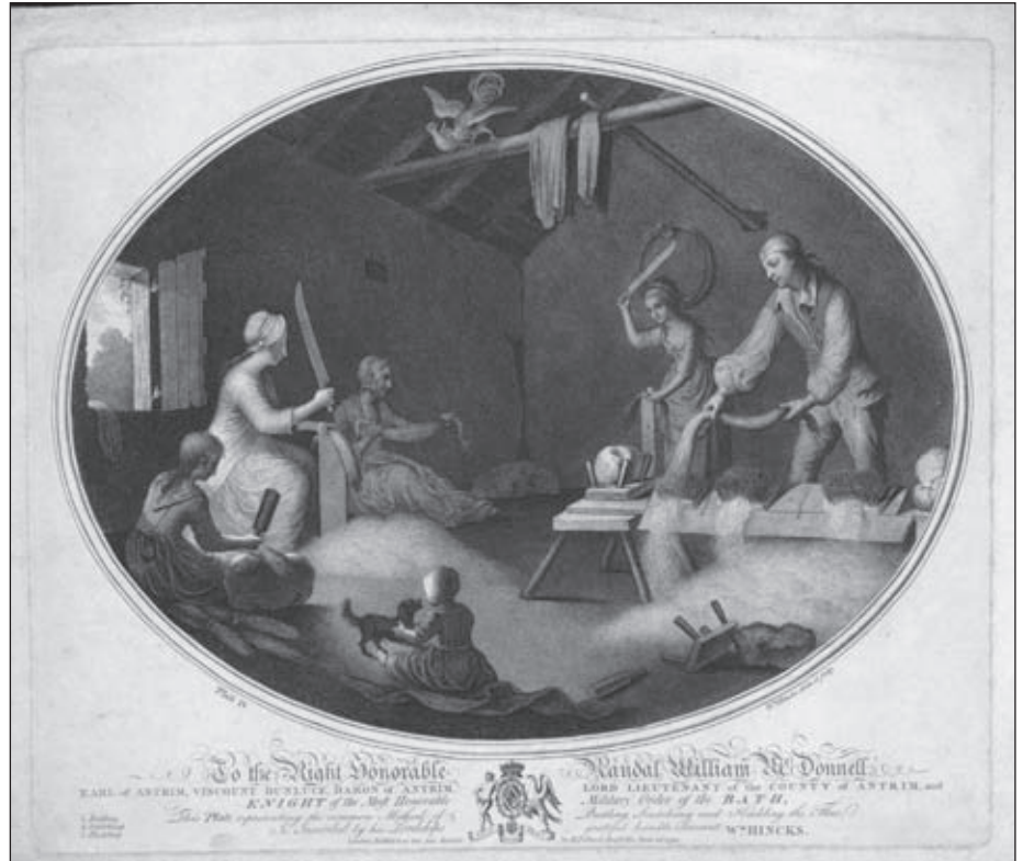
One of a celebrated set of engravings produced in 1791 by William Hincks showing aspects of linen production in Ireland. This plate is inscribed as illustrating 'the beetling, scutching and hackling of the flax'. Reproduced from the set in the Prints and Drawings Collection of the British Museum, London.
