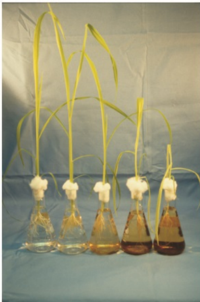
Figure 7.6 Examples of a laboratory whole sediment acute toxicity test conducted for 10 days with the infaunal amphipod, Ampelisca abdita , and phytotoxicity tests conducted with wetland plant seedlings such as the smooth cordgrass, Spartina alterniflora . Plants exposed for 21-28 days to either water-borne contaminants or contaminated whole sediment.
