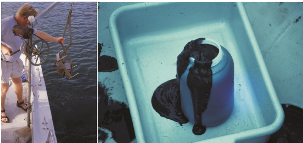
Figure 7.1 Contaminated sediment collected from Bayou Texar prior to analysis for chemical quality, toxicity, and benthic community composition. Sediment collected with a Petite ponar grab sampler to a depth of 13 cm or less.
