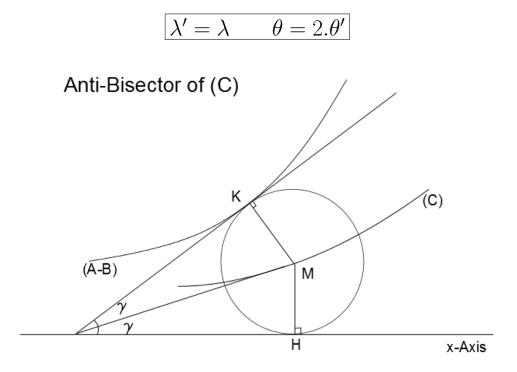
Figure 3: Anti-bisector of a curve (C) wrt x-axis.
