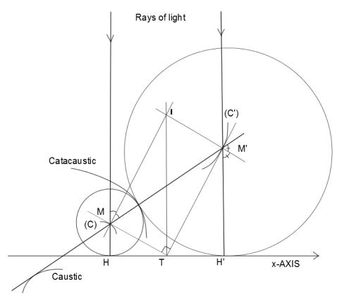
Orthogonal tangents transformation (OTT) : (C), (C'), Catacaustic and Caustic. The two curves (C) and (C') have the same anti-bissectante - the catacaustic -. The envelope of the line MM' is the caustic = the evolute of the catacaustic.
