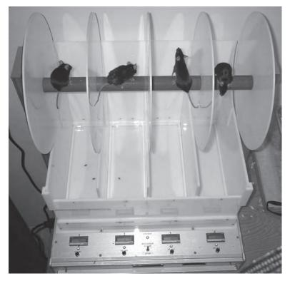
Fig 1 The Rotarod apparatus, showing four mice being tested, the circular dividers between compartments, the holding compartments, and timers for recording latency to fall.
