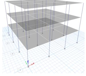
**Figure 1:** Finite Element Modelling of 3 Storey 3 Bay 4m Bay Length (3S3B4BLM2) Model
