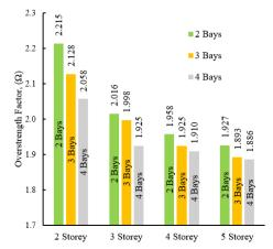
**Figure 3:** Overstrength factor for number of bay for various number of storey
