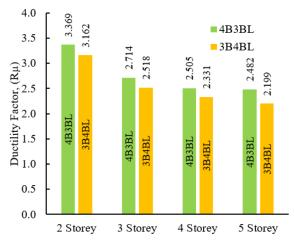
**Figure 9:** Ductility Factor for Model having Same Length (12m)
