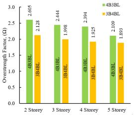
**Figure 5:** Overstrength Factor for Model having Same Length (12m)
