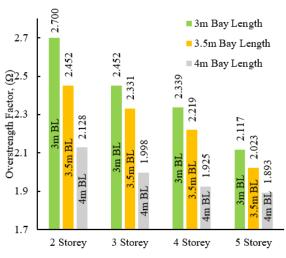
**Figure 4:** Overstrength factor for bay length for various number of storey
