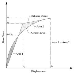
Figure 2: Bilinear Idealization of Pushover Curve
