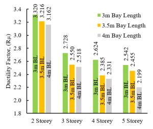
**Figure 8:** Ductility factor for bay length for various number of storey
