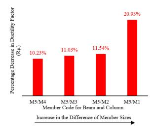
**Figure 10:** Effect on Ductility Factor by Difference in Member Sizes
