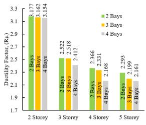
**Figure 7:** Ductility factor for number of bay for various number of storey
