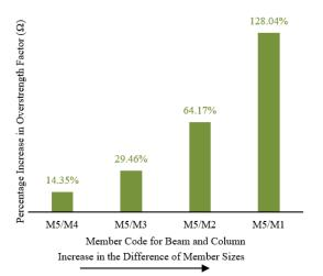
**Figure 6:** Effect on Overstrength Factor by Varying Member Sizes
