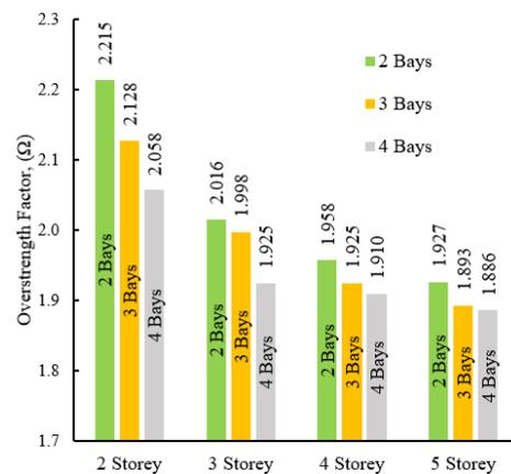
Figure 3: Overstrength factor for number of bay for various number of storey
