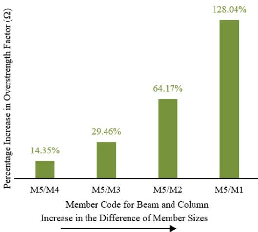
Figure 6: Effect on Overstrength Factor by Varying Member Sizes
