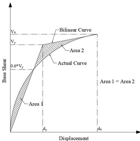
Figure 2: Bilinear Idealization of Pushover Curve
