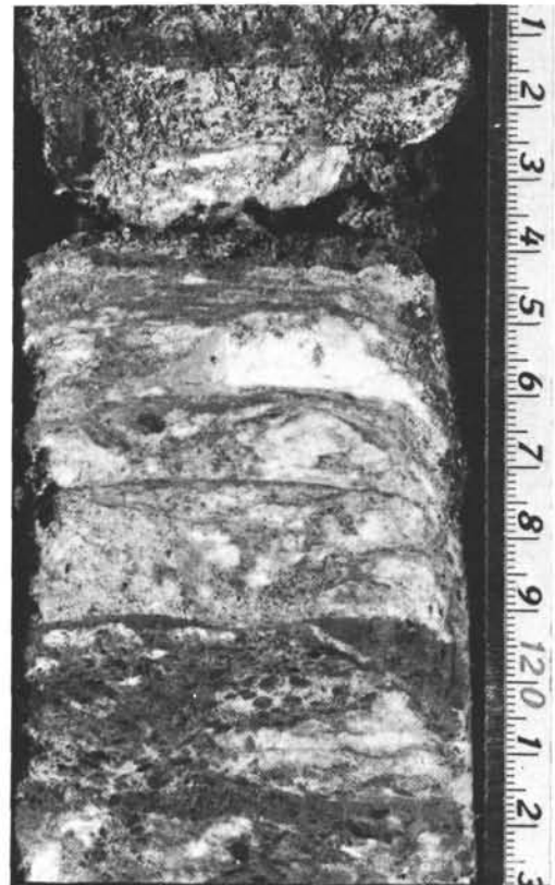
Figure 19. Laminated ( balatino ) facies of Core 10, Hole 134. The tiny white anhydrite spherules tend to form along the slightly coarser textured, darker dolomitic partings, and their penecontemporaneous growth often deforms the bedding interfaces.
