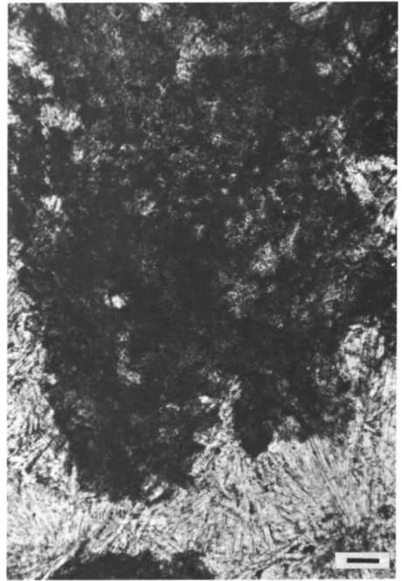
Figure 9. Concentration of semi-opaque, cryptocrystalline, probably organic-rich, matter in anhydrite. Site 124, Core 10, Section 1, Interval 53 to 55 cm. Scale bar represents 100 microns.
