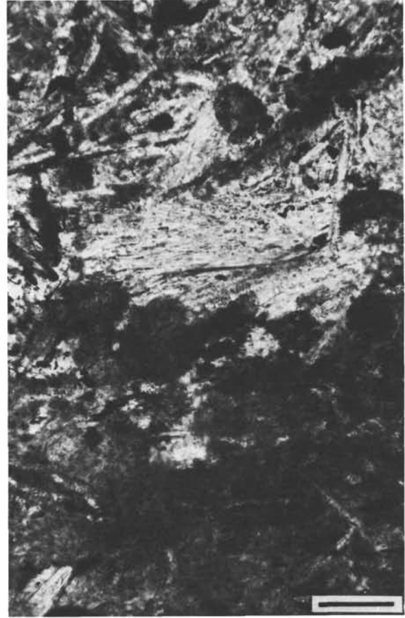
Figure 11. Anhydrite laths and dark, probably organic-rich in part, pelletlike material. Site 124, Core 9, Section 1, Interval 143 to 146 cm. Scale bar represents 100 microns.
