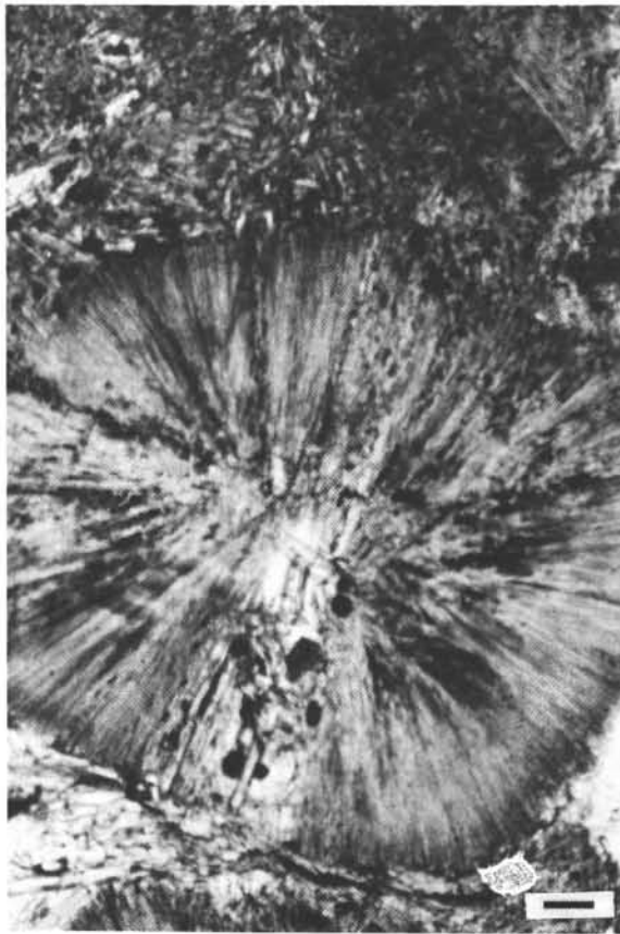
Figure 8. Anhydrite nodules with internodular lath-shaped anhydrite crystals. Site 124, Core 10, Section 1, Interval 53 to 55 cm. Scale bar represents 100 microns.
