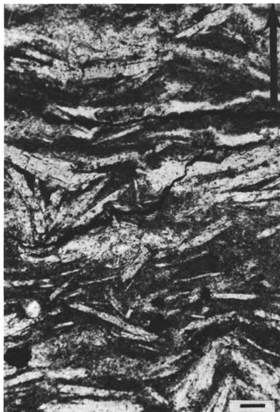
Figure 7. Couplets consisting of alternating anhydrite layers and dark gray semi-opaque, dolomite. Site 124, Core 10, Section 1, Interval 97 to 99 cm. Scale bar represents 100 microns; arrow indicates up.
