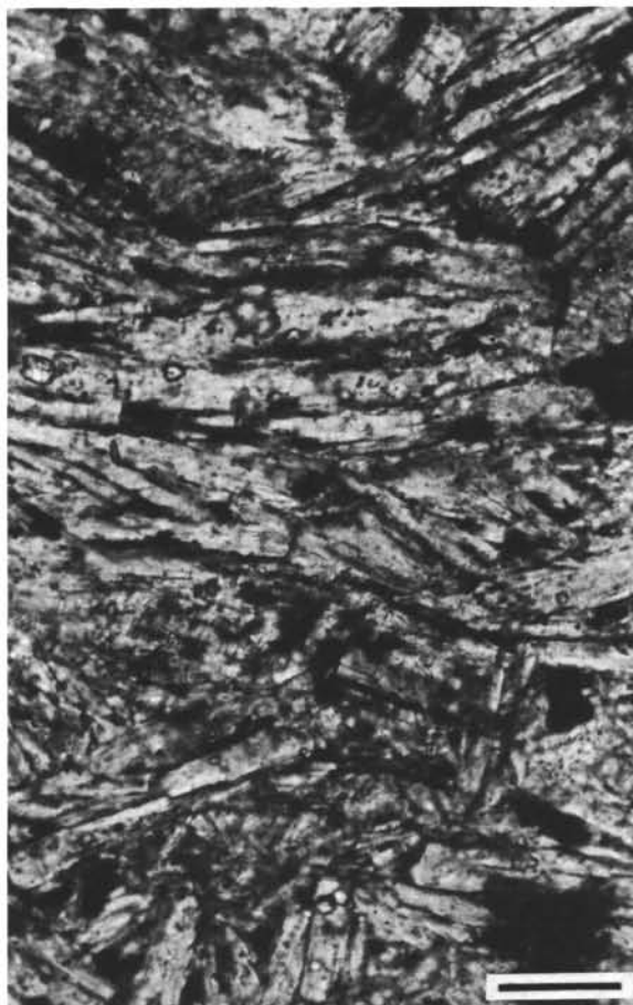
Figure 15. Anhydrite laths in subparallel orientation. Site 124, Core 9, Section 1, Interval 40 to 42 cm. Scale bar represents 100 microns.
