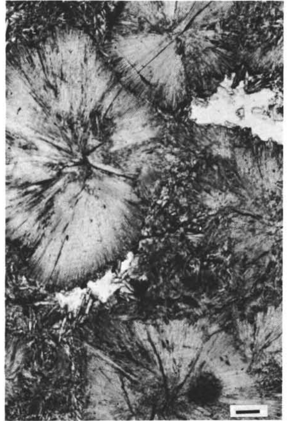
Figure 5. Anhydrite nodule with stellate arrangement of crystals. Site 124, Core 10, Section 1, Interval 53 to 55. Scale bar represents 100 microns.
