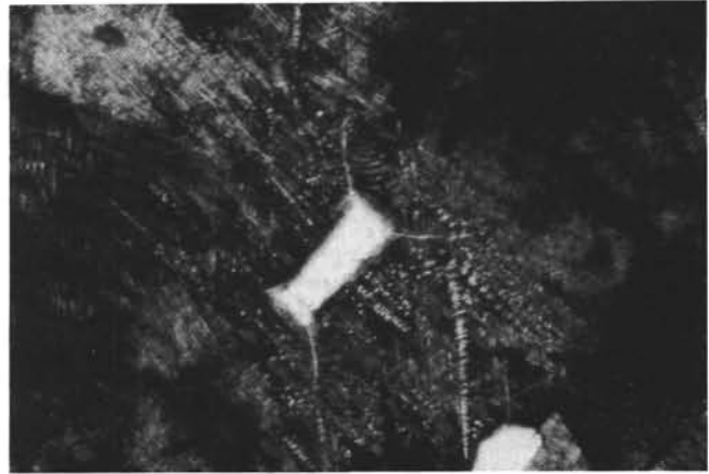
Figure 3. Reticulate olivine fibers and crystallites in glass matrix of SD-7B basalt. Scale = 25 \mu m.
