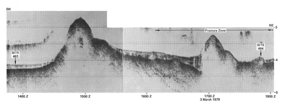
Figure 2. Seismic reflection profile recorded aboard *Glomar Challenger* between Sites 483 and 484 with an airgun sound source. (Vertical scale in seconds of two-way reflection time. Horizontal scale is given in time along ship's track. One hour represents about 10 km.)
