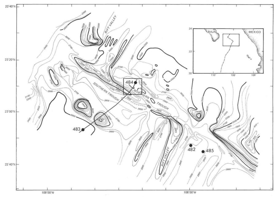
Figure 1. Bathymetric map of the Tamayo Fracture Zone showing general location of Site 484. Line connecting Sites 483 and 484 indicates location of *Challenger* profile shown in Figure 2. (Box around site shows position of detailed map presented in Fig. 3. Depths in m, corrected.)
