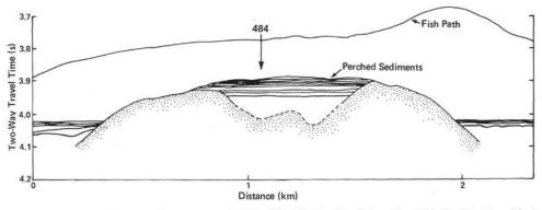
Figure 4. Cross section through the magnetic "diapir" drilled at Site 484 on Leg 65 (after MacDonald et al., 1979).
