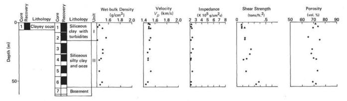
Figure 6. Sediment physical properties, Site 484. (Hole 484: triangles; Hole 484A: circles.)
