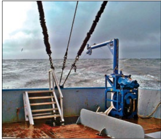
Figure 17. Sound-velocity measurements can be collected while the vessel is under way. Shown here is a deployed sound-velocity measuring device (a Brooke-Ocean Technology MVP-200) on the Anne S. Pierce over Georges Bank in the Atlantic Ocean. Courtesy of Timothy Kearns.
