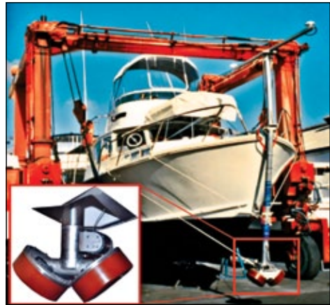
Figure 13. A dual-head multibeam echo sounder can be mounted on a retractable pole on the bow of a vessel, as shown here. Echo sounders are often mounted underneath the water line on the hull of the vessel adjacent to the keel. This Kongsberg EM3002D echo sounder can collect measurements from 0.5 meters to 150 meters. Courtesy of Kongsberg Maritime AS.
