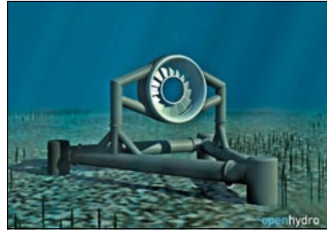
Figure 38. A schematic image of an open-center turbine designed to generate energy from underwater currents at the ocean floor. Courtesy of Open Hydro.
