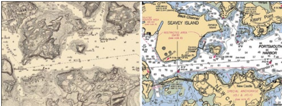
Figure 27. A historical chart of Portsmouth Harbor, New Hampshire (1866, 1:20,000), adjacent to a modern publication of the same chart (1980, 1:20,000). Soundings from the historical chart (in fathoms) closely match the measurements on the modern chart (in feet). Courtesy of NOAA.
