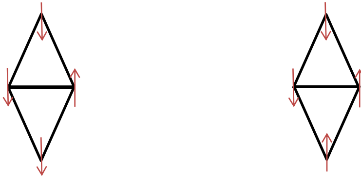
Fig. 11) represents two different arrangements of the Ising spin in the neighbouring triangles of the triangular lattice. Both the arrangements satisfy the equation 1.9. Even after fixing the spin arrangement of upper triangle, the spin at lower triangle can arrange itself in 2 ways. [26]
