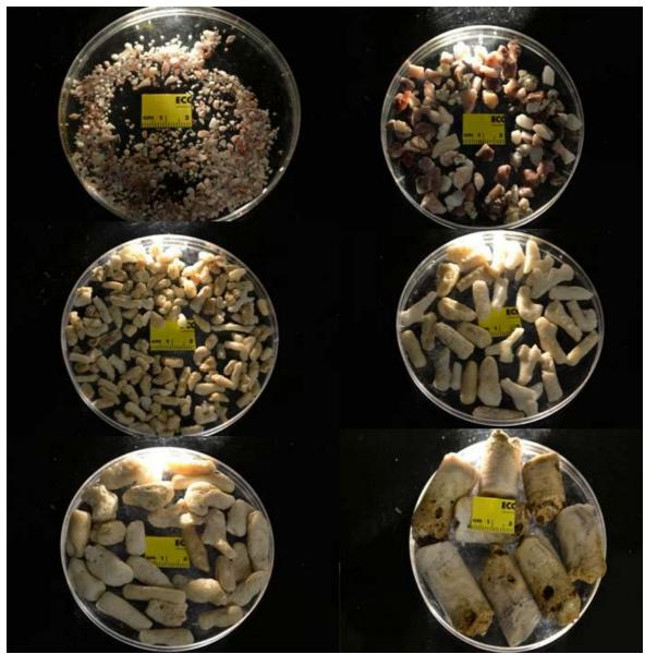
Figure 1. Different grades of calcite (top two) and aragonite (bottom four) used in the adsorption and leaching experiments. One of the aragonite samples (bottom left) was excluded from data analysis due to an unforeseen loss of liquid during the adsorption phase (i.e. the author is a klutz and broke a sample bottle).
