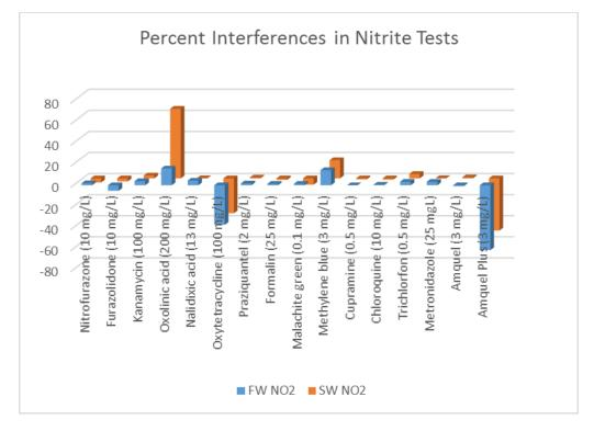
Figure 2: Interference levels in nitrite tests (as  $NO_2^{-}$ ) by percent difference.
