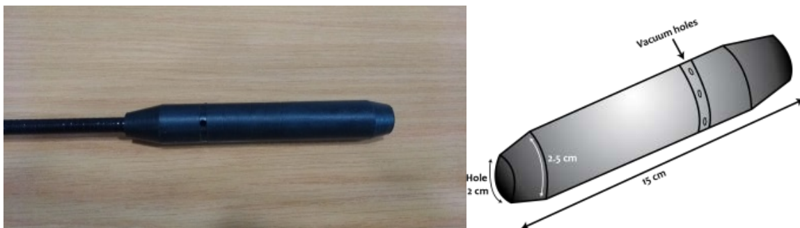
Figure 2. a) Machined HDPE chamber mounted on carbon spear shaft. B) Chamber details and dimensions.
