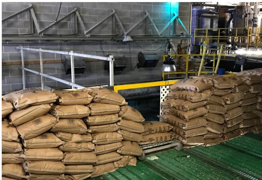
**Figure 4.** Five pallets worth of salt were staged around the tank's perimeter and in the adjacent areas. Plastic lattice work was used to prevent salt bags from prematurely falling into the tank.
