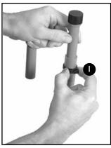
Attach 2 each Suction Cup Clamps H with 2 each Suction Cups G to the Inlet Pipe C so that it can be secured to the aquarium.
