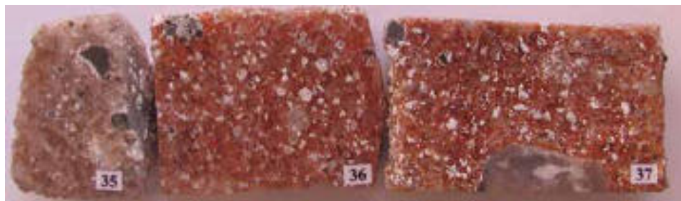
Fig. 7. Rock salt (halite) with anhydrite inclusions (light and grey). Core sample from the Omega Parametric Borehole. The sample is about 5 cm wide.
