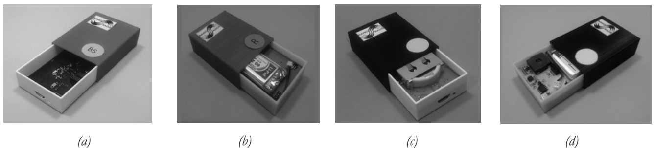
Fig. 2. Nodes of active UWB network based on universal module: base station (a); relay node (b); active RFID tag (c); acoustic sensor node (d).
