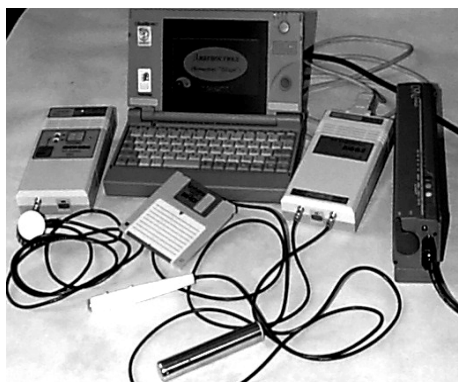
Therapeutic-diagnostic complex "Charm" for electropuncture express diagnostics and EHF-therapy (option with autonomous power supply).
