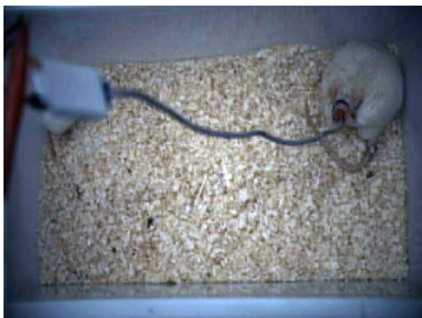
Fig. 2. The EEG cable connecting the head of the rat with the EEG signal amplifier, randomly moves in the field of view of the video camera. The case of the amplifier closed the image of the young male, which resulted in loss of video capture.
