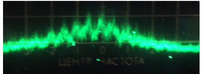
Fig. 8. The total spectrum of the reflected signal with the reference signal on the screen C4-60 (scanning scales -50 MHz/div).
