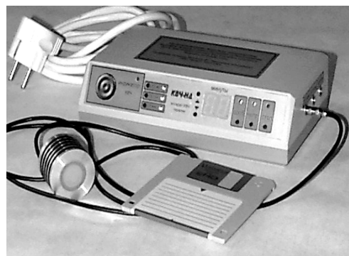
The device "KVCH-ND" for three frequency ranges 7.1: 5.6 and 4.9 mm for puncture EHF-therapy.
