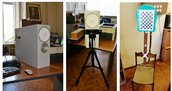
Fig. 3. An experimental setup that includes a passive terahertz receiver (a), a time-of-flight camera (b) and a calibration board (c).
