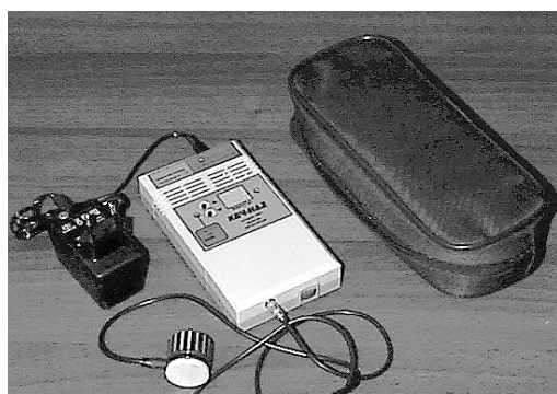
Apparatus "KVCH-ND2" of the new generation with autonomous power for puncture EHF-therapy (wearable version).
