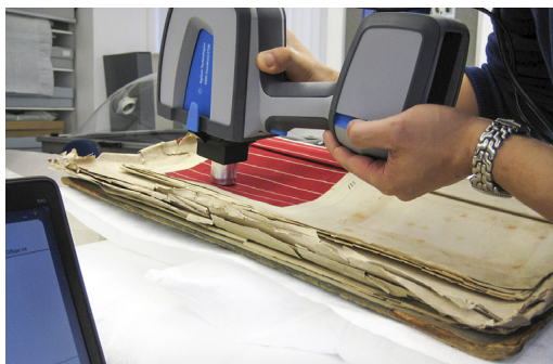
Figure 2. DRIFTS analysis of 18th-century Turkey red (UGD 13/8/2) at the CTC with Dr Leung Tang
