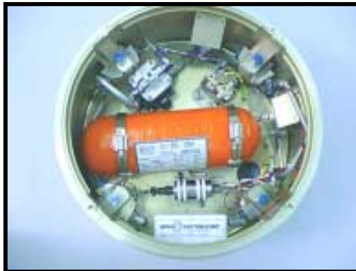
Figure I.4-1: Pneumatic subsystem, rate sensor, battery
