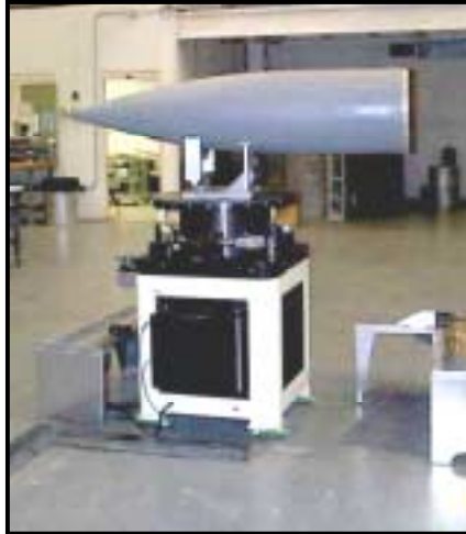
Figure 7.2.1-1 Airdyne Mark 8 Mass Properties Measurement System at WFF
