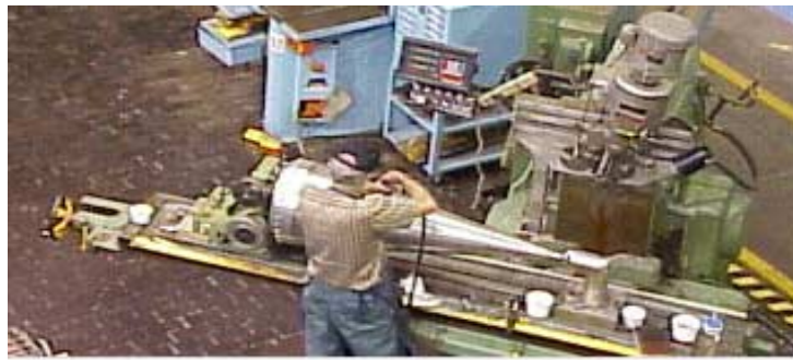
Figure 11.1.4-2: A Nose Cone is Streamlined in the Machine Shop
