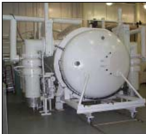
Figure 7.2.4-1 PV/T Vacuum Chamber (left) and Tenney Space Simulation Thermal Vacuum Chamber at WFF
