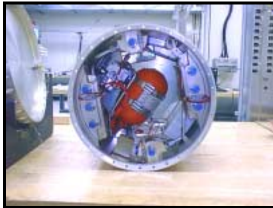
Figure I.5-1: Pneumatic Subsystem = Reservoir, Regulator, Valves And Transducer
