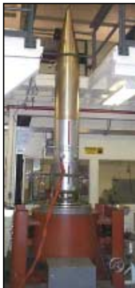
Figure 7.2.3-1 Ling Electronics B335 Thrust Axis Shaker at WFF
