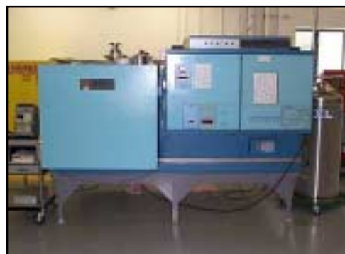
Figure 7.2.4-1 PV/T Vacuum Chamber (left) and Tenney Space Simulation Thermal Vacuum Chamber at WFF
