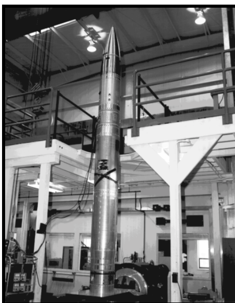
Figure 11.1.3-1. Astrophysics Payload (36.022) undergoing Lateral Vibration Testing
