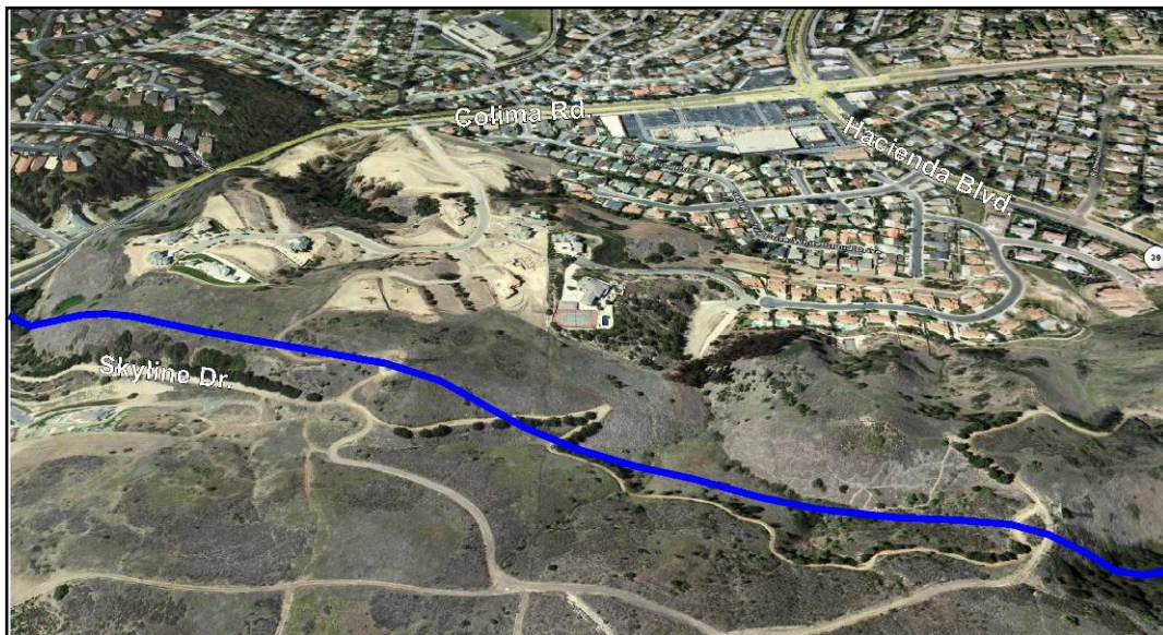
Photo 18: Aerial (oriented north) of potential portal exit location east of Colima Road in Hacienda Heights, accessible from Skyline Drive (~S8A MP 9.8). The blue line indicates the proposed T/L route paralleling existing 220-kV T/Ls. Source: Google Earth
