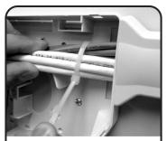
Secure the cables to the 4 base using the cable tie anchor points. Route cables through appropriate outlet locations in the base.
