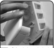
Defeat the bottom latches by 1 pulling up on the bottom of the cover at the seam and remove the cover.
