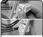
Insert CT couplers into the 5b appropriate opening and push until it snaps into place.
