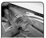
Align the tray into position 7 and push the center latch down to lock the tray to the base. Be careful not to pinch fibers.
