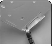
Using wire cutters, remove 2 the appropriate breakout position for cable/raceway entry.
