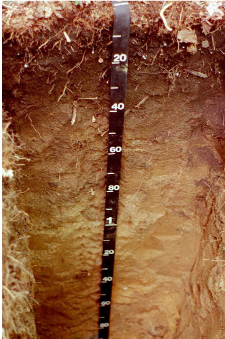
Figure 40.—Profile of Tanasee soil series near Purchase Knob in Great Smoky Mountains National Park. Scale is in centimeters.
