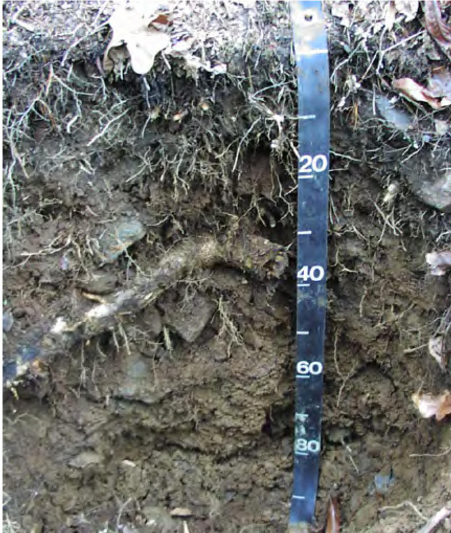
Figure 39.—Profile of Sylco soil series in Great Smoky Mountains National Park. Scale is in centimeters.
