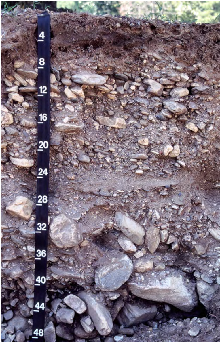
Figure 38.—Profile of Potomac soil series (outside Great Smoky Mountains National Park). Scale is in inches.
