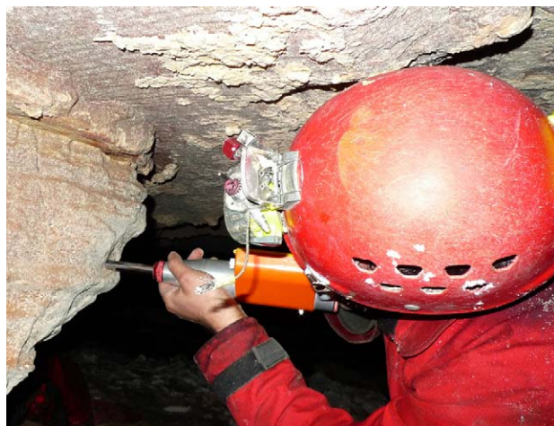
Fig. 45: Field measurements of rock hardness by Schmidt hammer in Cueva Juliana.
