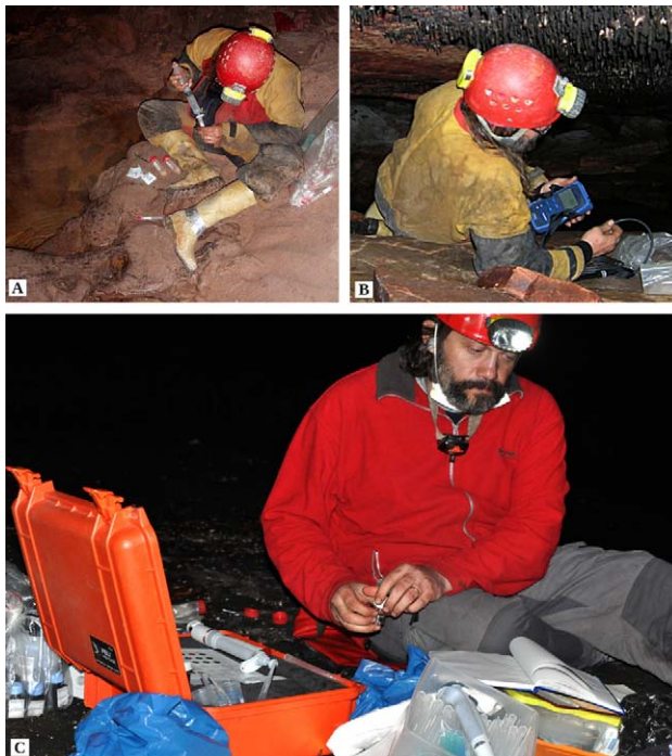
Fig. 36: Hydrogeochemical field work. A – Water sampling and filtering through a 0.45 µm mesh in Cueva Charles Brewer, Churí Tepui. B – Measurement of the pH and electrical conductivity in water samples, Cueva Ojos de Cristal, Roraima. C – Colorimetric analyses in the Northern Camp, Churí Tepui.
