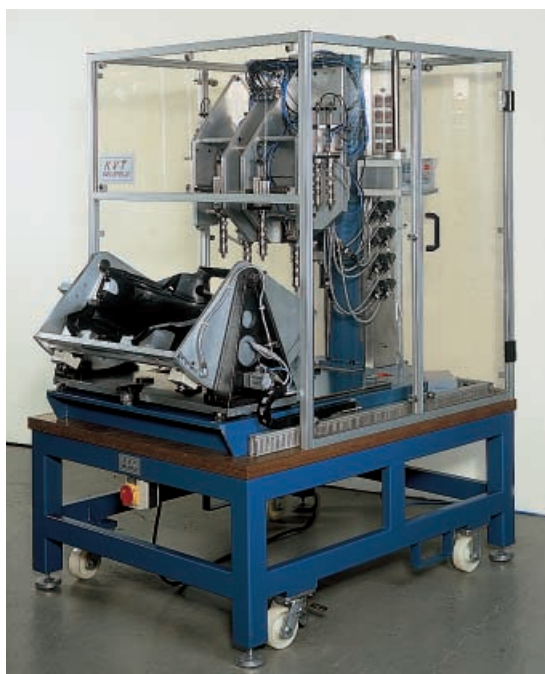
10-item thermal installation (HES) semi-automatic
